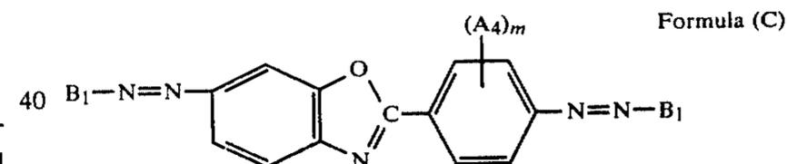
wherein  $B_1$  represents a coupler residue and  $A_4$  is a hydroxyl or an acylamino group when  $m$  is an integer of 1 to 4, or also an alkoxy group when  $m$  is an integer of 2 to 4.
