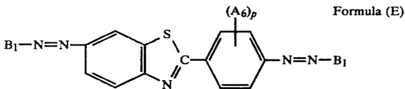
wherein B<sub>1</sub> represents a coupler residue, A<sub>6</sub> is a hydrogen atom, a halogen atom, a lower alkyl, a lower alkoxy, an acylamino or a hydroxyl group, and p is an integer of 1 to 4.
