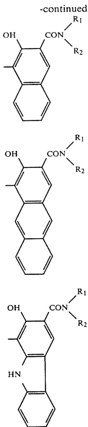
wherein  $R_1$  is a hydrogen atom, an unsubstituted or substituted alkyl, or an unsubstituted or substituted phenyl group and  $R_2$  is an unsubstituted or substituted alkyl, or an unsubstituted or substituted aryl group.
