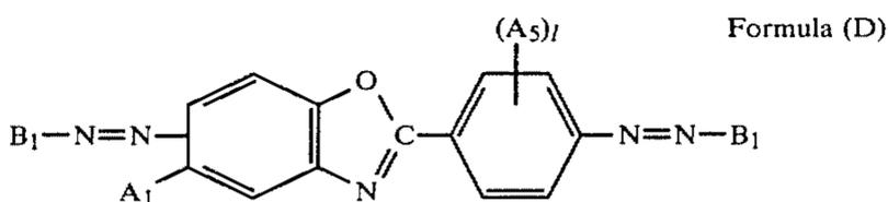
wherein B<sub>1</sub> represents a coupler residue, A<sub>1</sub> is methyl or chlorine, A<sub>5</sub> a hydrogen atom, a halogen atom, a lower alkyl, a lower alkoxy, an acylamino or a hydroxyl group, and l an integer of 1 to 4.
