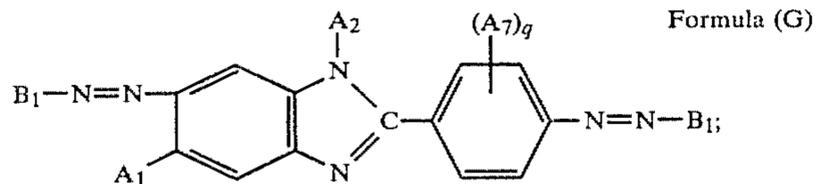
wherein  $B_1$  represents a coupler residue,  $A_1$  is a lower alkyl group,  $A_2$  is a lower alkyl group,  $A_7$  is a hydrogen atom, a halogen atom, a lower alkyl, a lower alkoxy, an acylamino or a hydroxyl group, and  $q$  is an integer of 1 to 4.
