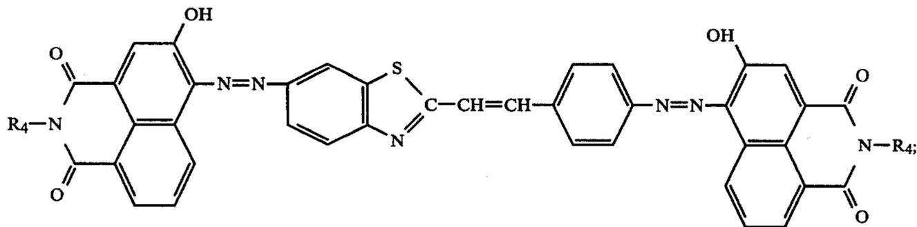
wherein R<sub>4</sub> is an unsubstituted or substituted alkyl, or an unsubstituted or substituted phenyl group.
