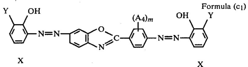
wherein  $A_4$  is a hydroxyl or an acylamino group when  $m$  is an integer of 1 to 4, or also an alkoxy group when  $m$  is an integer of 2 to 4,  $X$  is an atomic group forming a naphthalene-, anthracene-, carbazole- or dibenzofuran-ring together with the benzene ring, and  $Y$  a group of the formula
