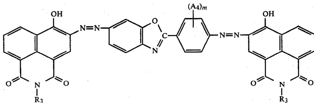
wherein  $A_4$  is a hydroxyl or an acylamino group when  $m$  is an integer of 1 to 4, or also an alkoxy group when  $m$  is an integer of 2 to 4 and  $R_3$  is an unsubstituted or substituted alkyl, or an unsubstituted or substituted phenyl group.
