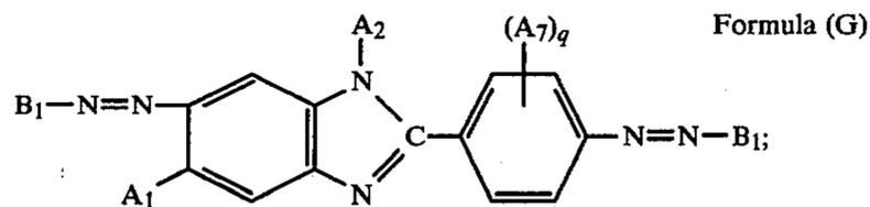
wherein B<sub>1</sub> represents a coupler residue, A<sub>1</sub> is a lower alkyl group, A<sub>2</sub> is a lower alkyl group, A<sub>7</sub> is a hydrogen atom, a halogen atom, a lower alkyl, a lower alkoxy, an acylamino or a hydroxyl group, and q is an integer of 1 to 4.
