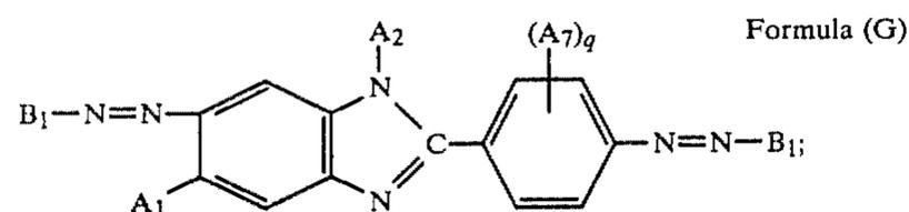
wherein  $B_1$  represents a coupler residue,  $A_1$  is a lower alkyl group,  $A_2$  is a lower alkyl group,  $A_7$  is a hydrogen atom, a halogen atom, a lower alkyl, a lower alkoxy, an acylamino or a hydroxyl group, and  $q$  is an integer of 1 to 4.
