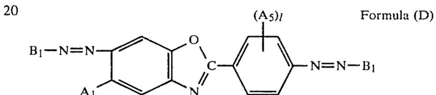
wherein B<sub>1</sub> represents a coupler residue, A<sub>1</sub> is a lower alkyl group or a halogen atom, A<sub>5</sub> is a hydrogen atom, a halogen atom, a lower alkyl, a lower alkoxy, an acylamino or a hydroxyl group, and l is an integer of 1 to 4.
