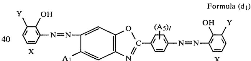
wherein A<sub>1</sub> is a lower alkyl group, or a halogen atom, A<sub>5</sub> is a hydrogen atom, a halogen atom, a lower alkyl, a lower alkoxy, an acylamino or a hydroxyl group; l is an integer of 1 to 4, X is an atomic group forming a naphthaleneanthracene-, carbazole- or dibenzofuran-ring together with the benzene ring, and Y is a group of the formula
