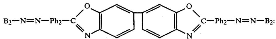
wherein Ph<sub>2</sub> is an unsubstituted or substituted phenylene group and B<sub>2</sub> is a coupler residue.
