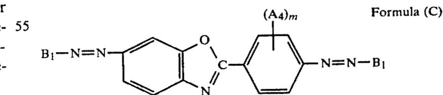
wherein  $B_1$  represents a coupler residue and  $A_4$  a hydroxyl or an acylamino group when  $m$  is an integer of 1 to 4, or also an alkoxy group when  $m$  is an integer of 2 to 4.
