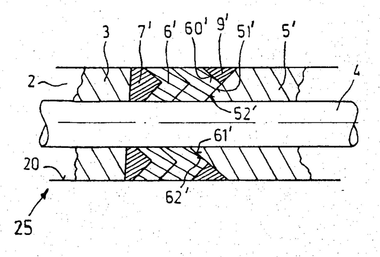
APPARATUS FOR SEALING A HIGH PRESSURE INSTALLATION INCLUDING A MOVABLE MEMBER, ESPECIALLY AN OSCILLATORY MOVABLE PLUNGER OR A ROTARY SHAFT
