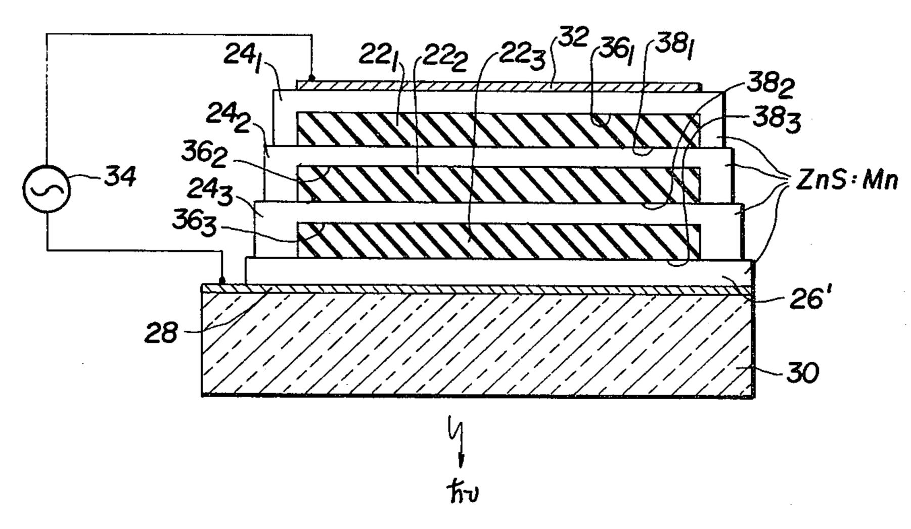
electroluminescent devices which exhibit an enhanced resistance to failure.
