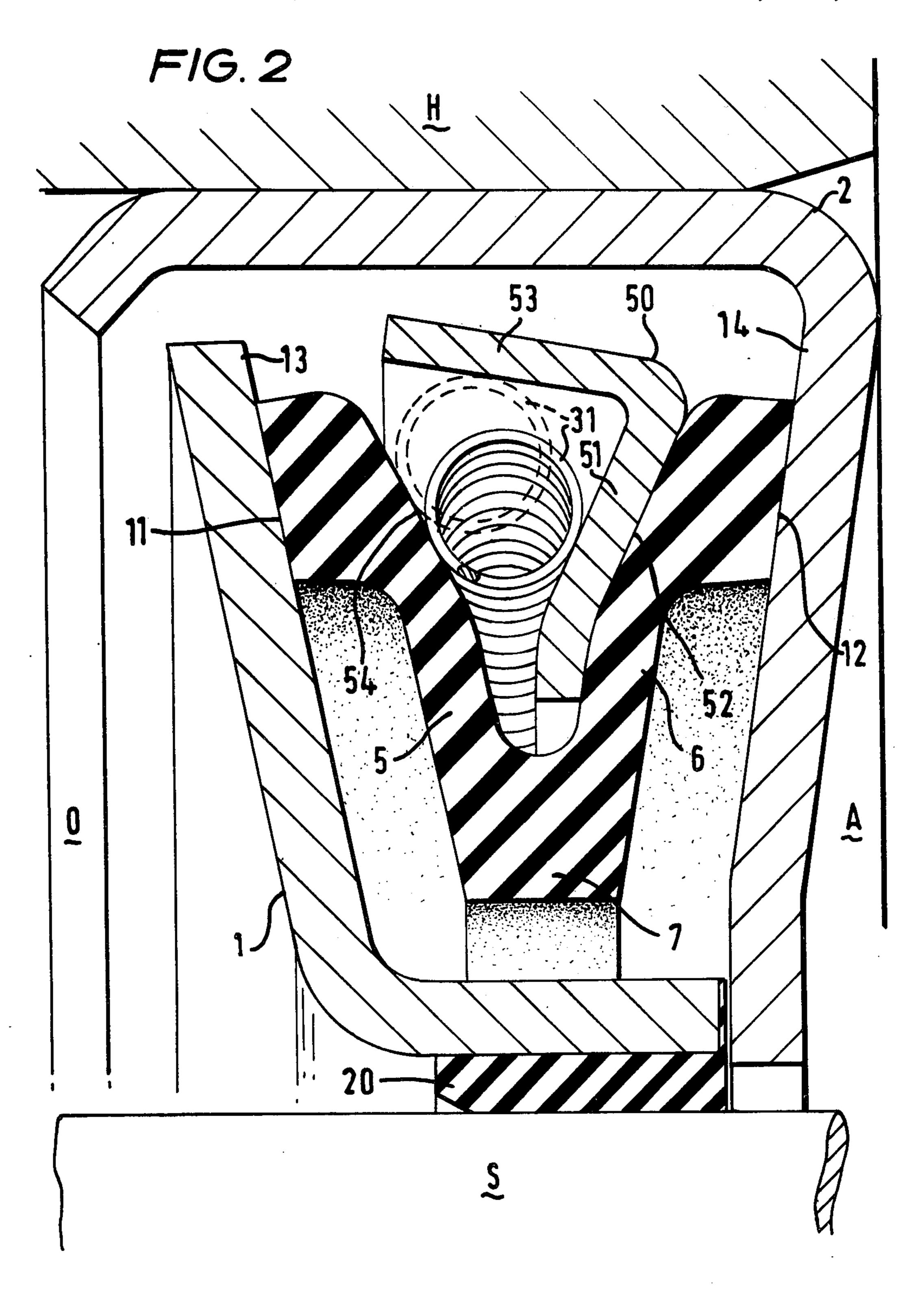
bear on their counterfaces sufficiently for the ring 7 to be entrained in rotation but, for speeds up to about 1000 RPM for a ring of 140 mm outer diameter, the speed of rotation of the ring 7 is not likely to be so high that the
