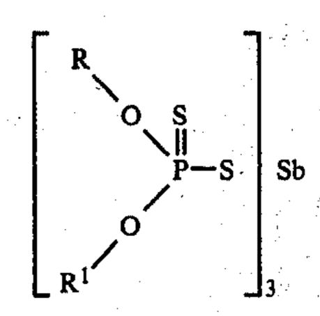
wherein R and R' can be the same or different and are hydrocarbyl radicals containing from 1 to 18 carbon atoms.
