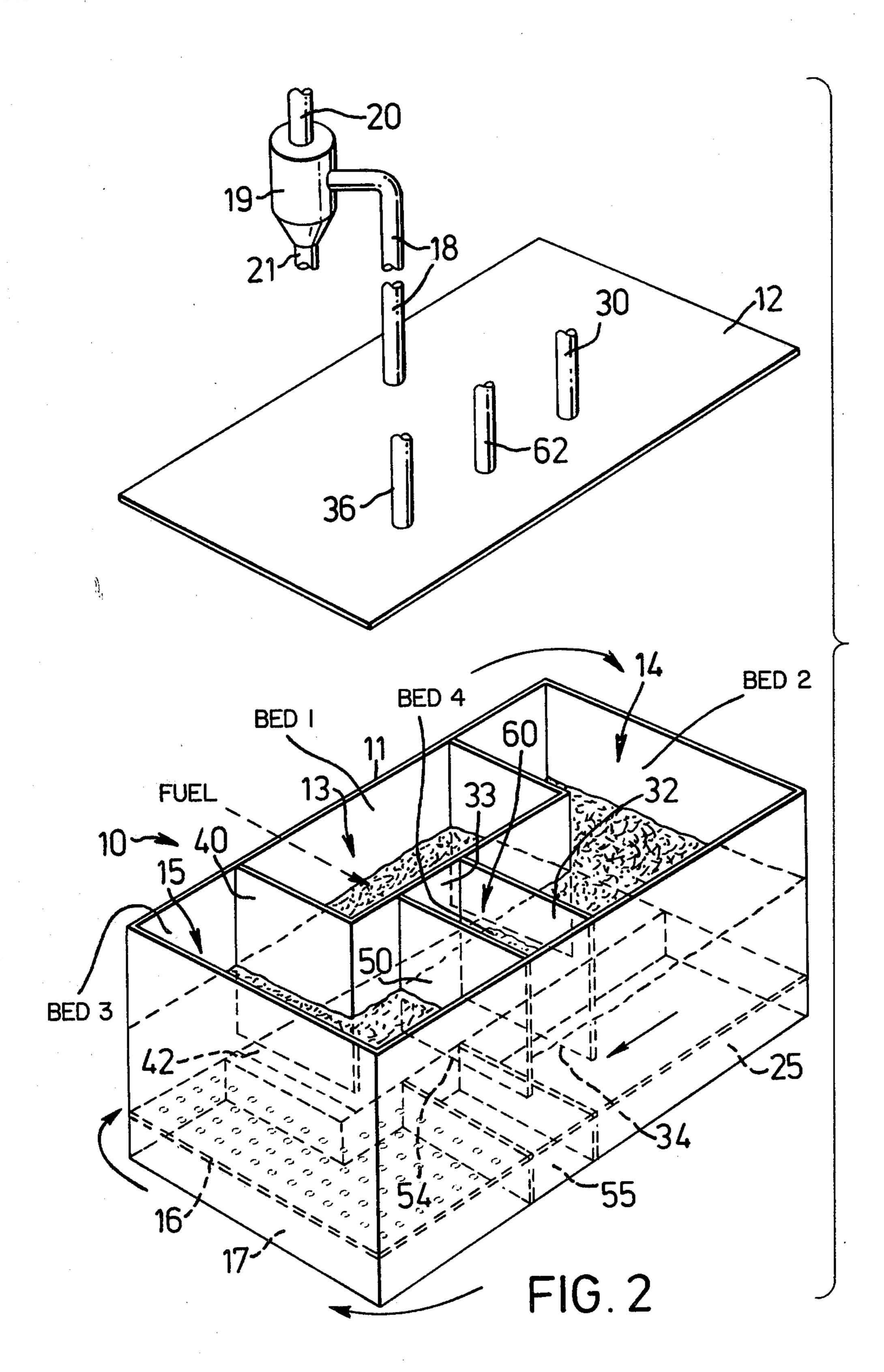
APPARATUS FOR CONVERTING A FUEL TO COMBUSTIBLE GAS
