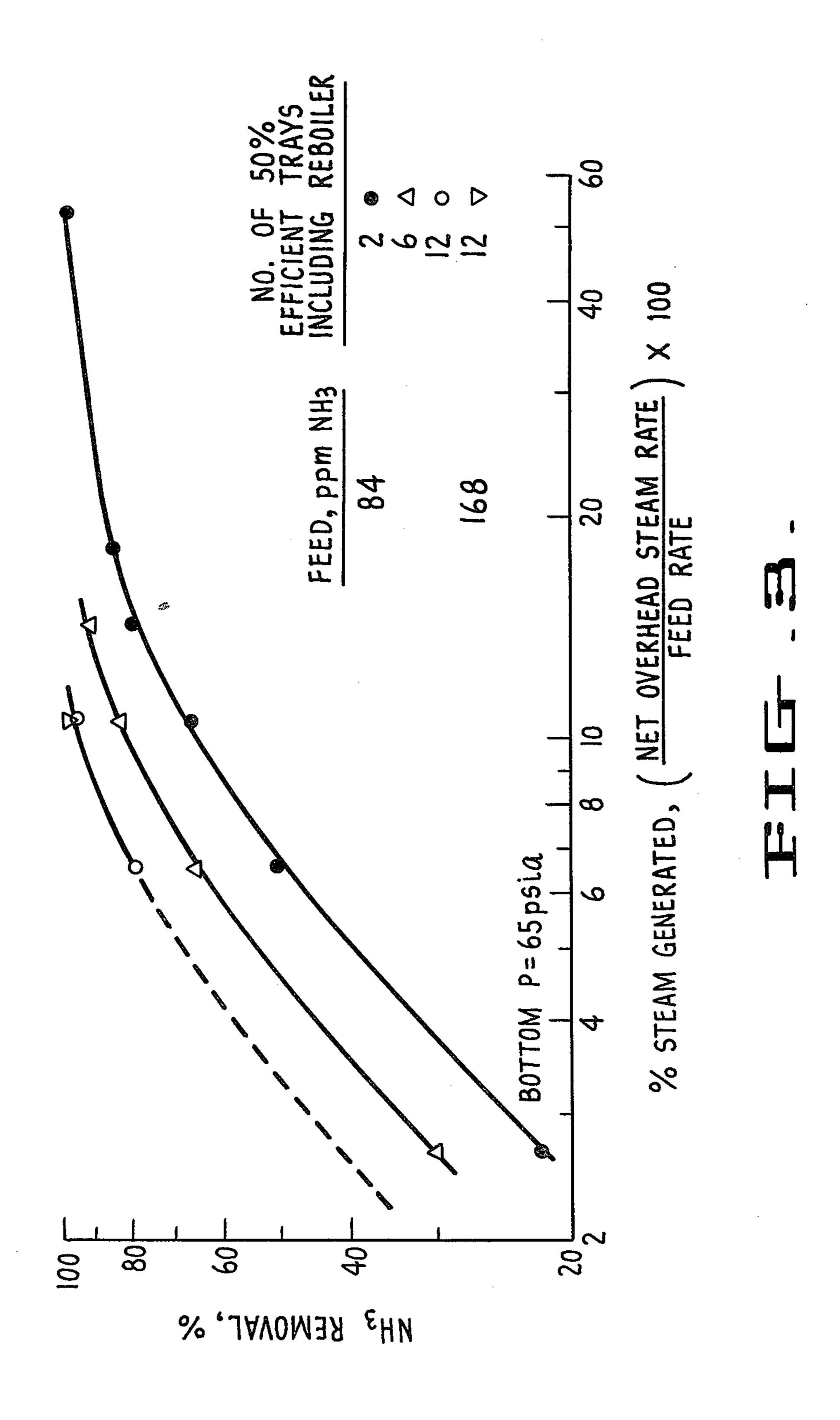
FIG. 3 is a graph setting forth ammonia removal efficiencies as a function of stripper column tray count and overhead fraction.
