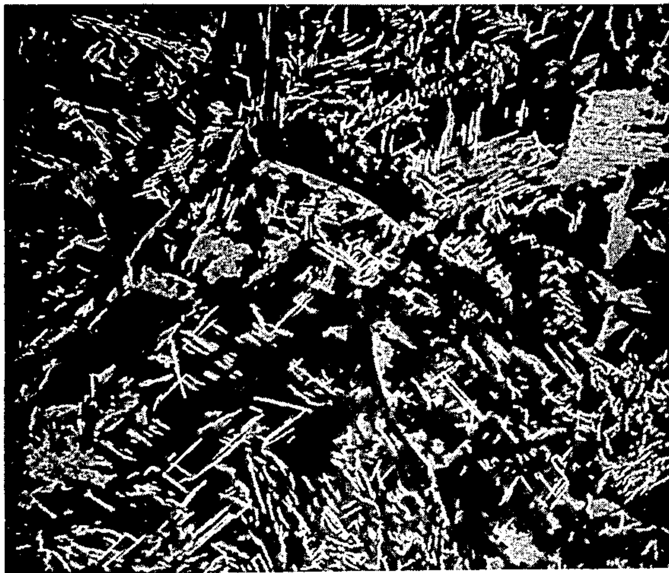
AS RECEIVED 6150 SEM 2000X PICRAL HEAT G
