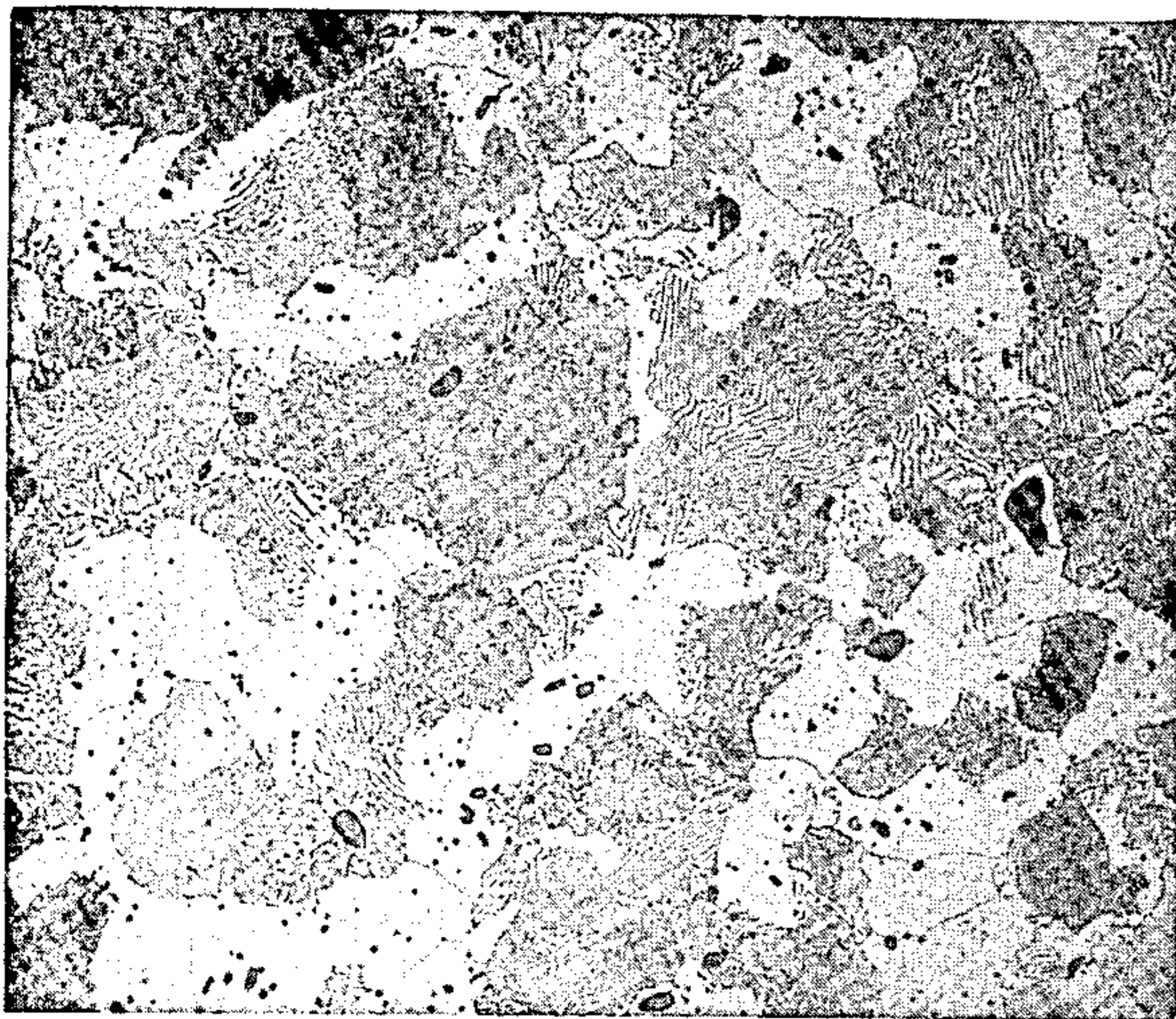
FURNACE ANNEALED 1144 LIGHT METALLOGRAPH 500X PICRAL HEAT H
