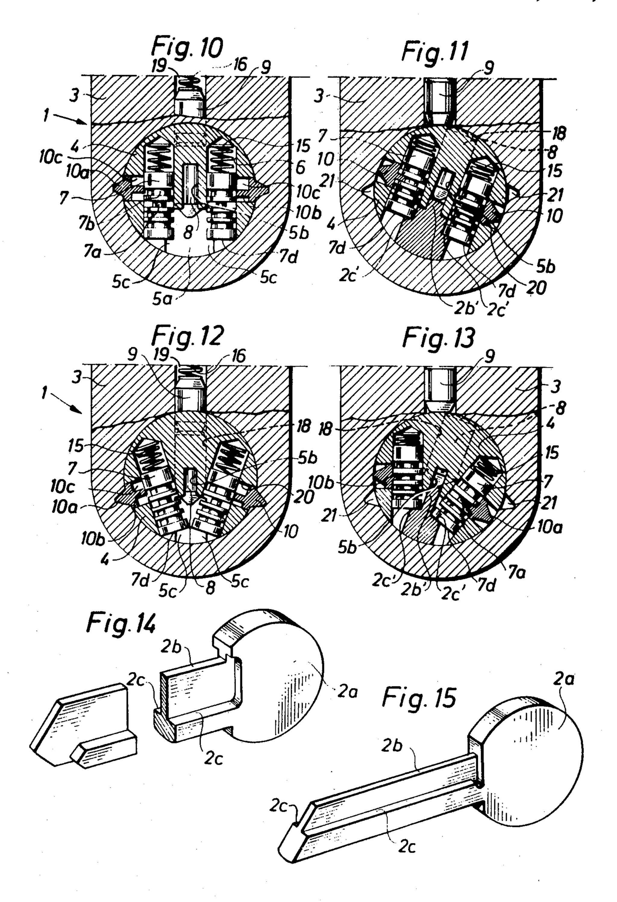
METHOD OF MANUFACTURING A KEY FOR A CYLINDRICAL LOCK
