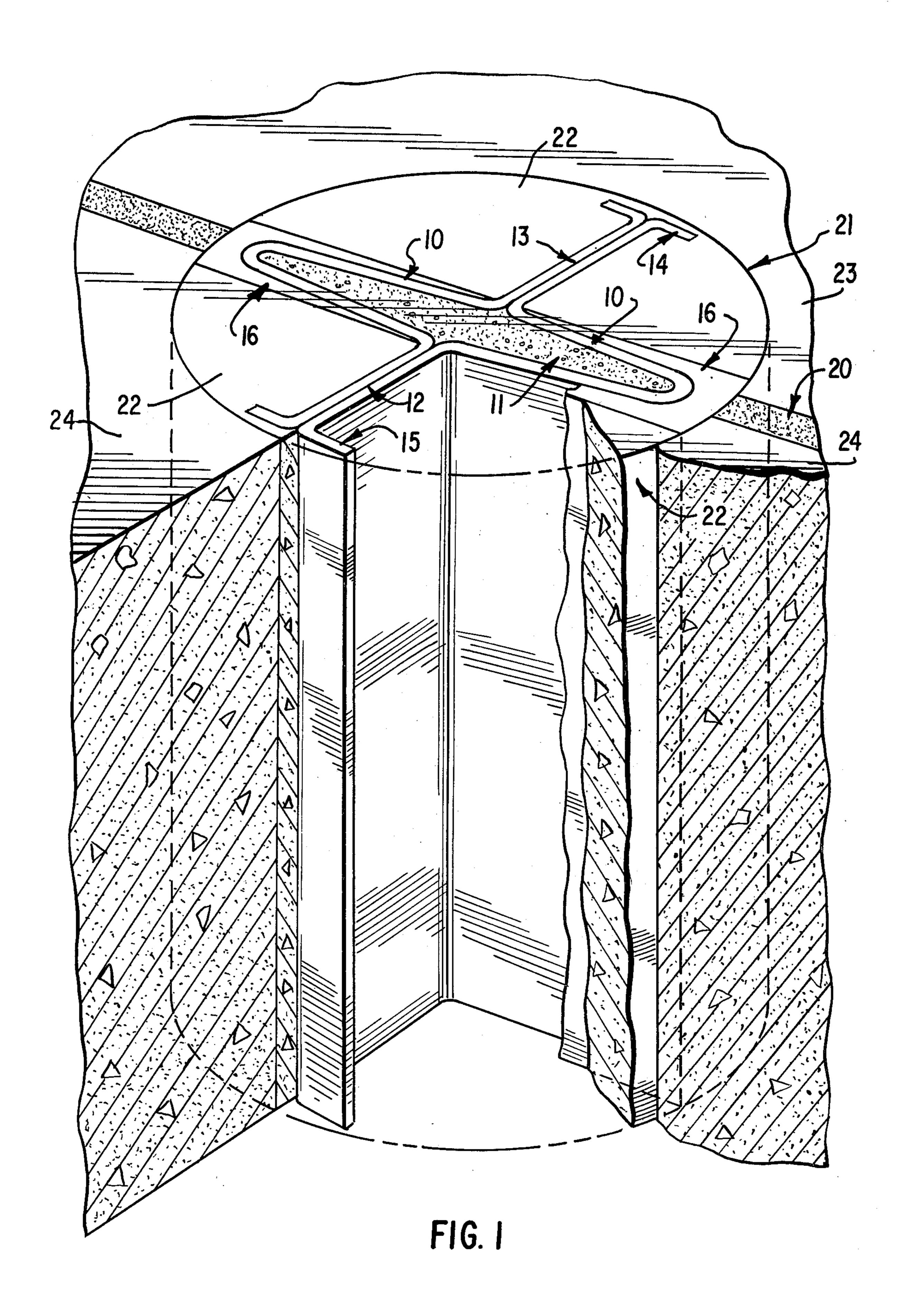
LOAD TRANSFER DEVICE FOR JOINTS IN **CONCRETE SLABS**
