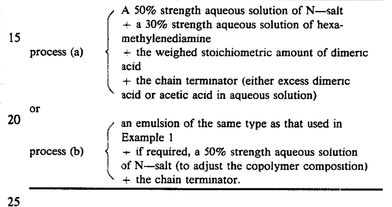
The apparatus was purged with nitrogen and the temperature of the mixture was then raised to 225° C. while maintaining the autogenous pressure. A pressure of 20 bars was reached. Water was distilled under pressure for 1 hour, so as to impart a high temperature to the mixture, namely  $\theta$ °C. The distillation was stopped in order to carry out the homogenization stage, lasting x minutes at  $\theta$ °C. material temperature, under P bars water vapor pressure.
