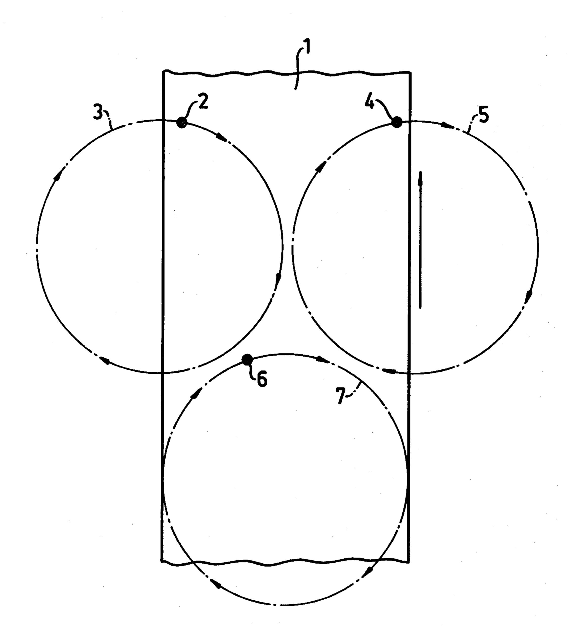
METHOD AND APPARATUS TO DETECT RANDOMLY DISTRIBUTED DISCONTINUITIES IN DIFFERENT DIRECTIONS IN A LONGITUDINALLY MOVING WEB USING ROTATING PROBES IN OVERLAPPED PATHS
