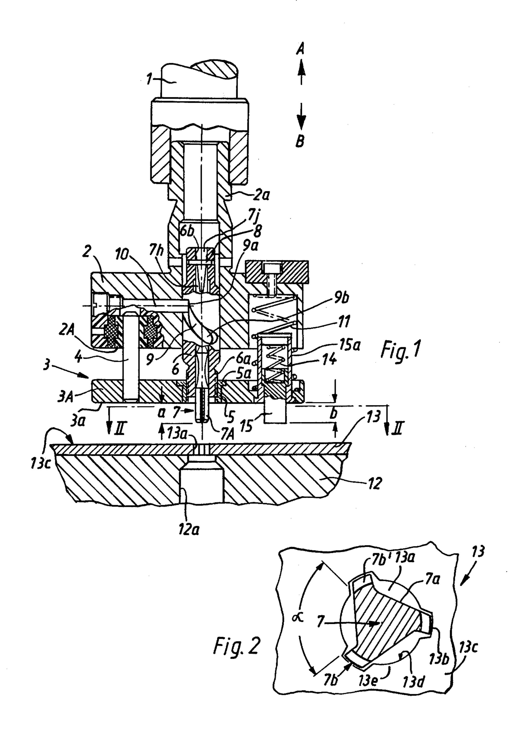
tapping hole when the thread cutting operation is com-
