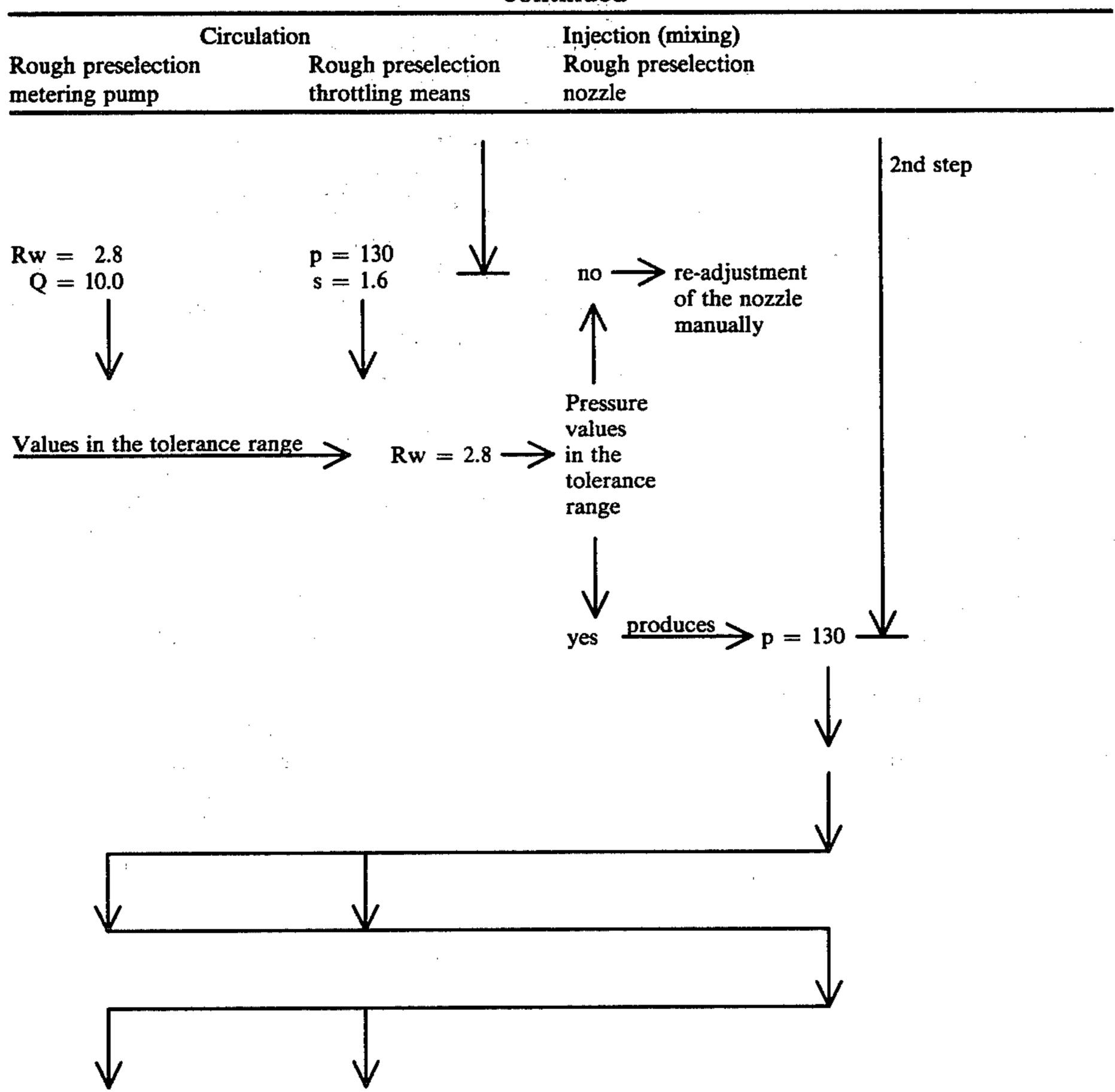
As shown by the circulation control steps, a value of Q=10.0 kg/min and p=148 bar, which lies within the permitted deviations, has been adjusted after the 4th control step.
