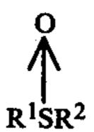
where R<sup>1</sup> and R<sup>2</sup> are substituents having between 1 and 12 carbon atoms. A preferred hydrogen sulfide scrubber embodiment the reduced sulfide species produced from the corresponding sulfoxide is reoxidized and recirculated to scrub more fuel gas.
