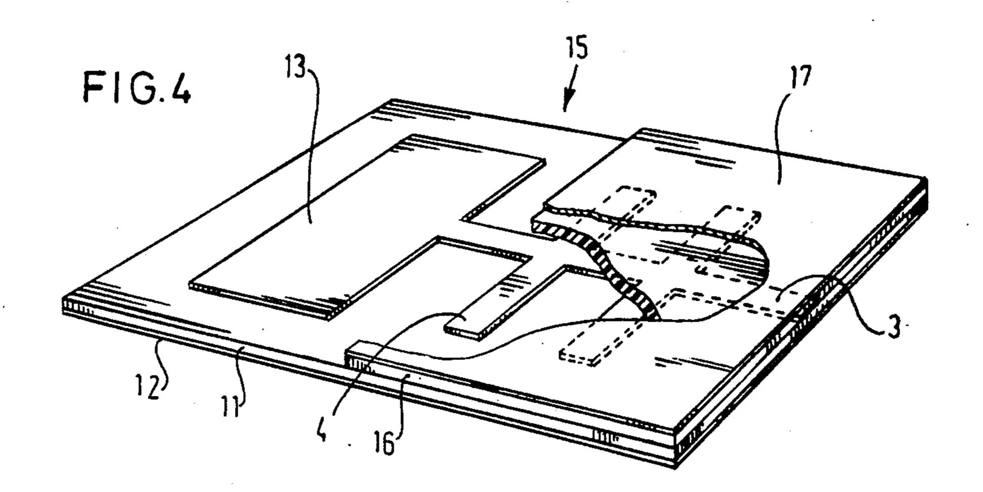
The invention has for its object to construct a resonator antenna of the type described in a manner such that a relative bandwidth of about 5 to 10% can be attained, while maintaining the desired radiation properties.
