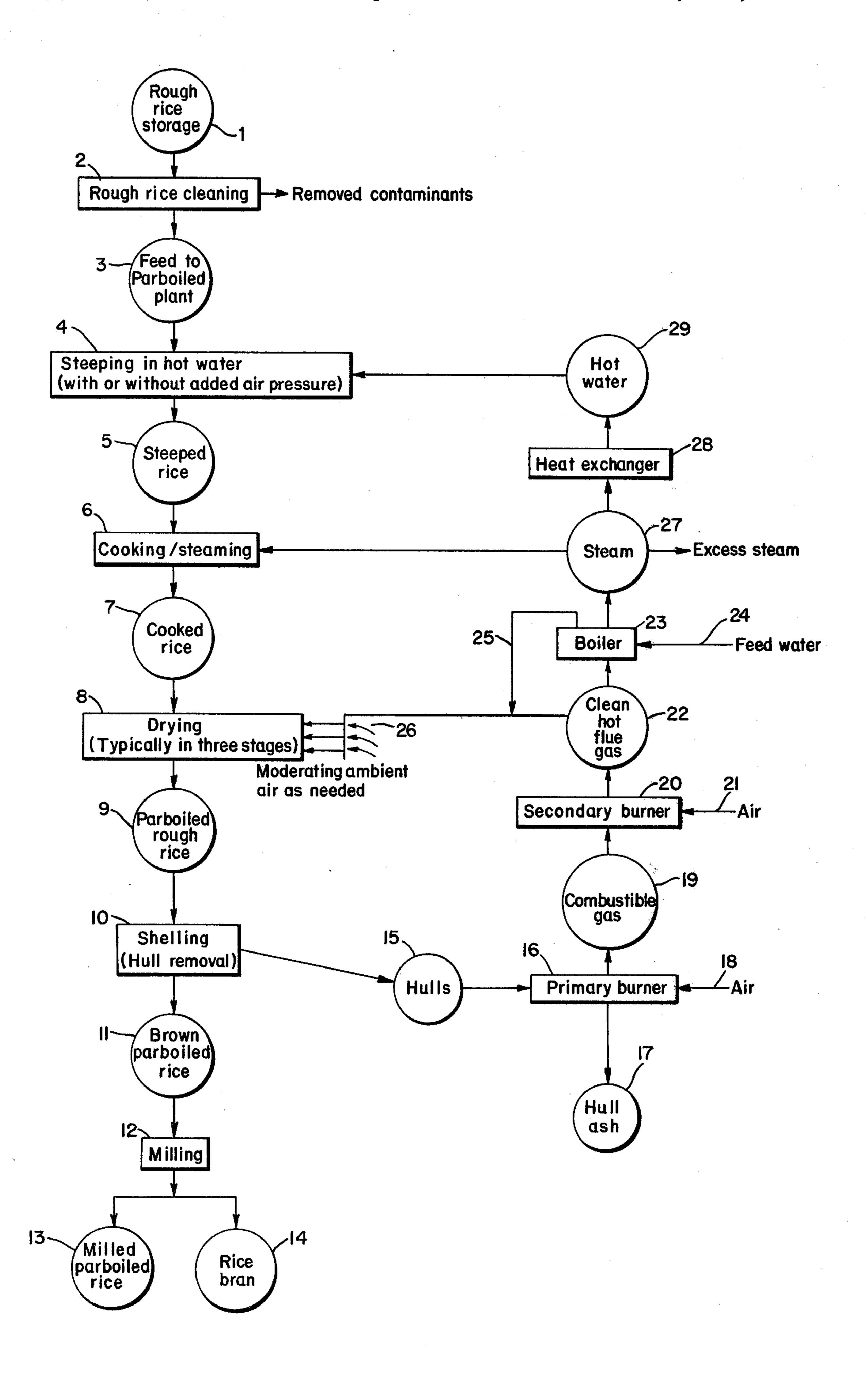
recirculated into the system to provide heat for the rice
