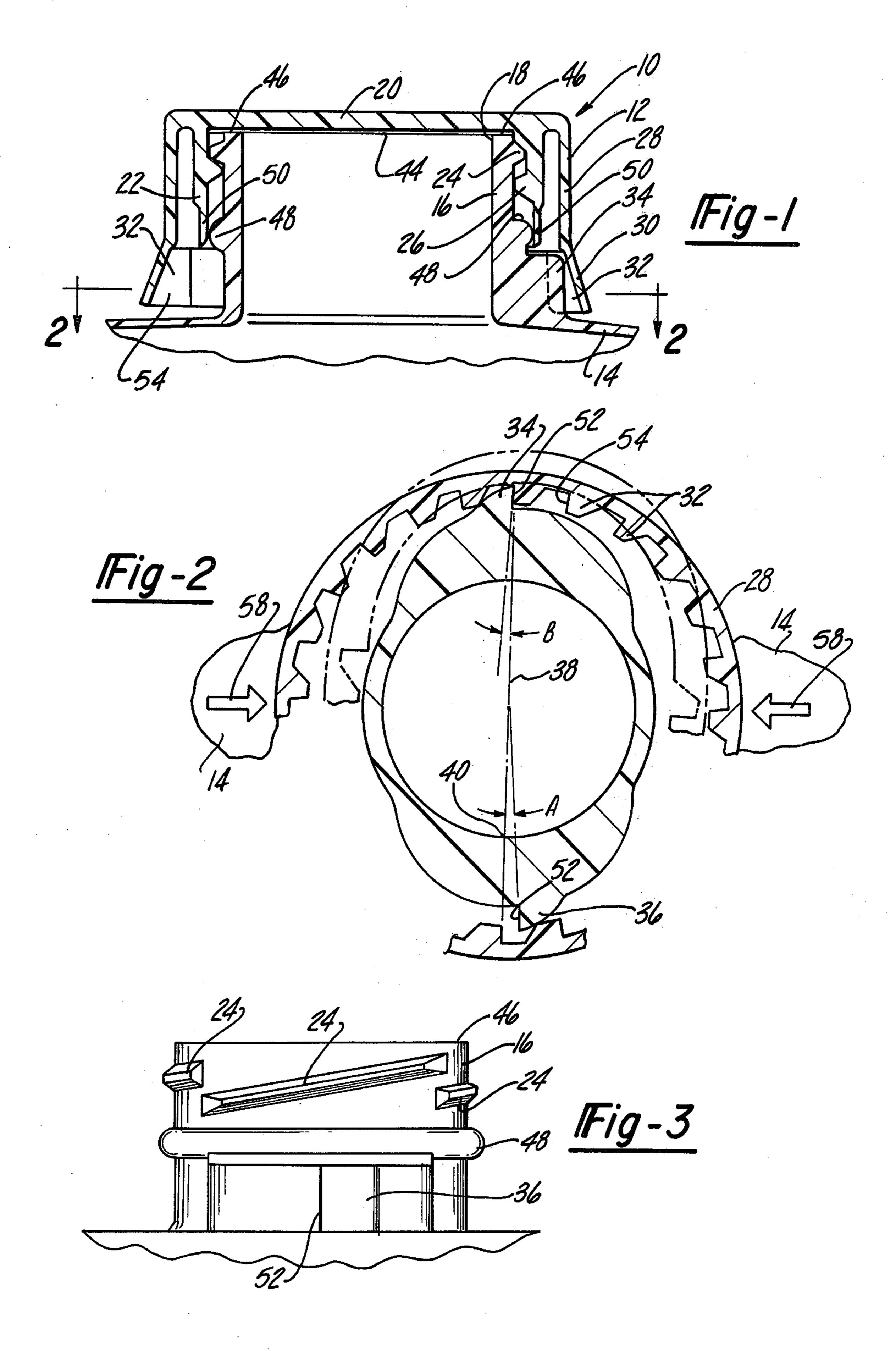
elements is engaged with one of the plurality of teeth on the closure.
