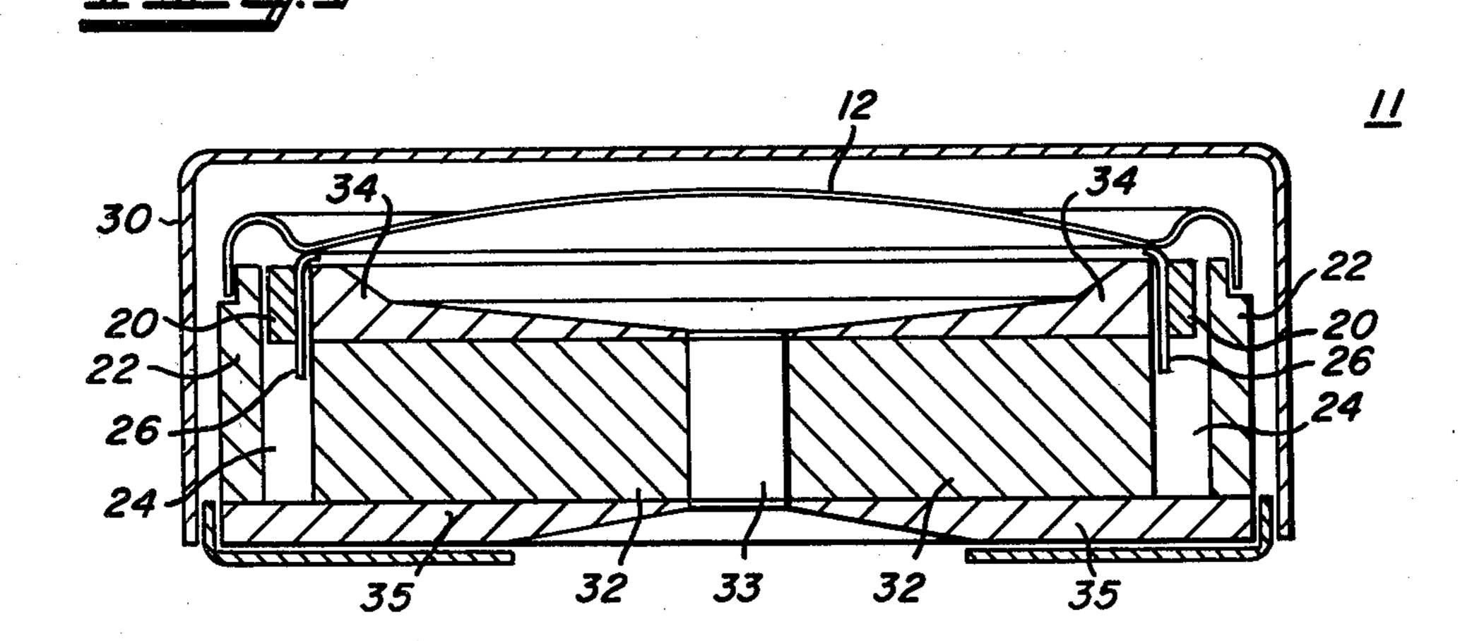
ACOUSTICAL TRANSDUCER WITH A SLOTTED PISTON SUSPENSION
