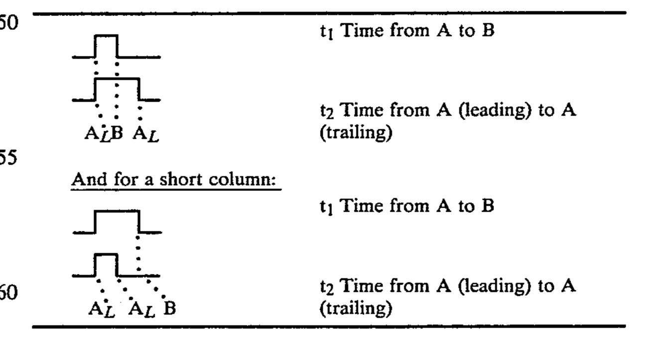
If D is the distance from photodetector A to photodetector B and t<sub>1</sub> is the time required for the leading edge of a liquid column to travel from A to B then velocity is
