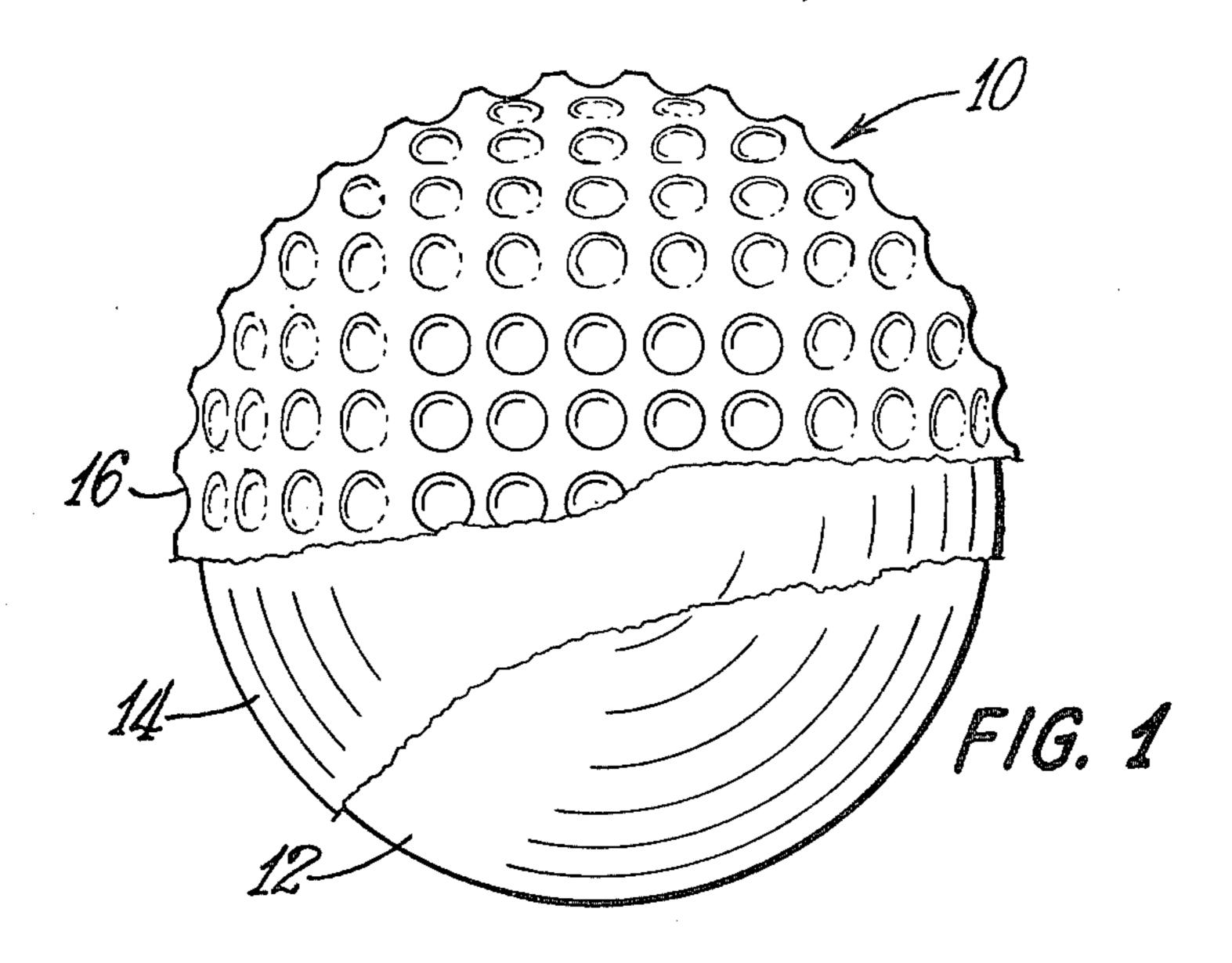
14 LAYER OF CELLULAR OR NON-CELLULAR HARD, HIGH FLEXURAL MODULUS RESINOUS MATERIAL OF A THICKNESS IN A RANGE OF .020 AND .070 INCHES
