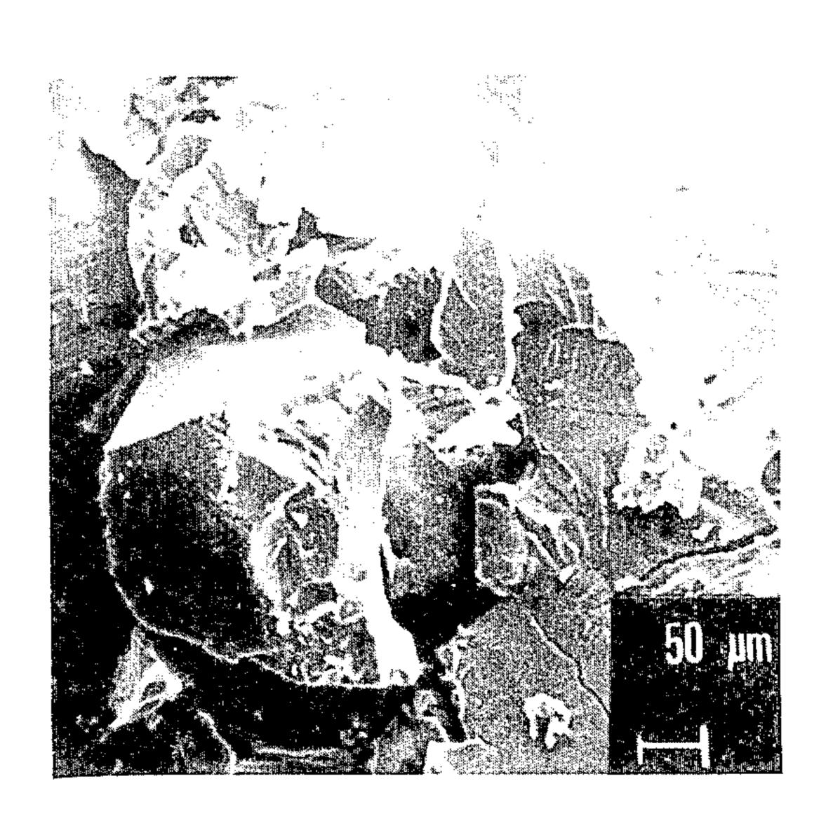
FIG. 4 Electron micrograph of 100%SBR tire rubber, cryogenically crushed.
