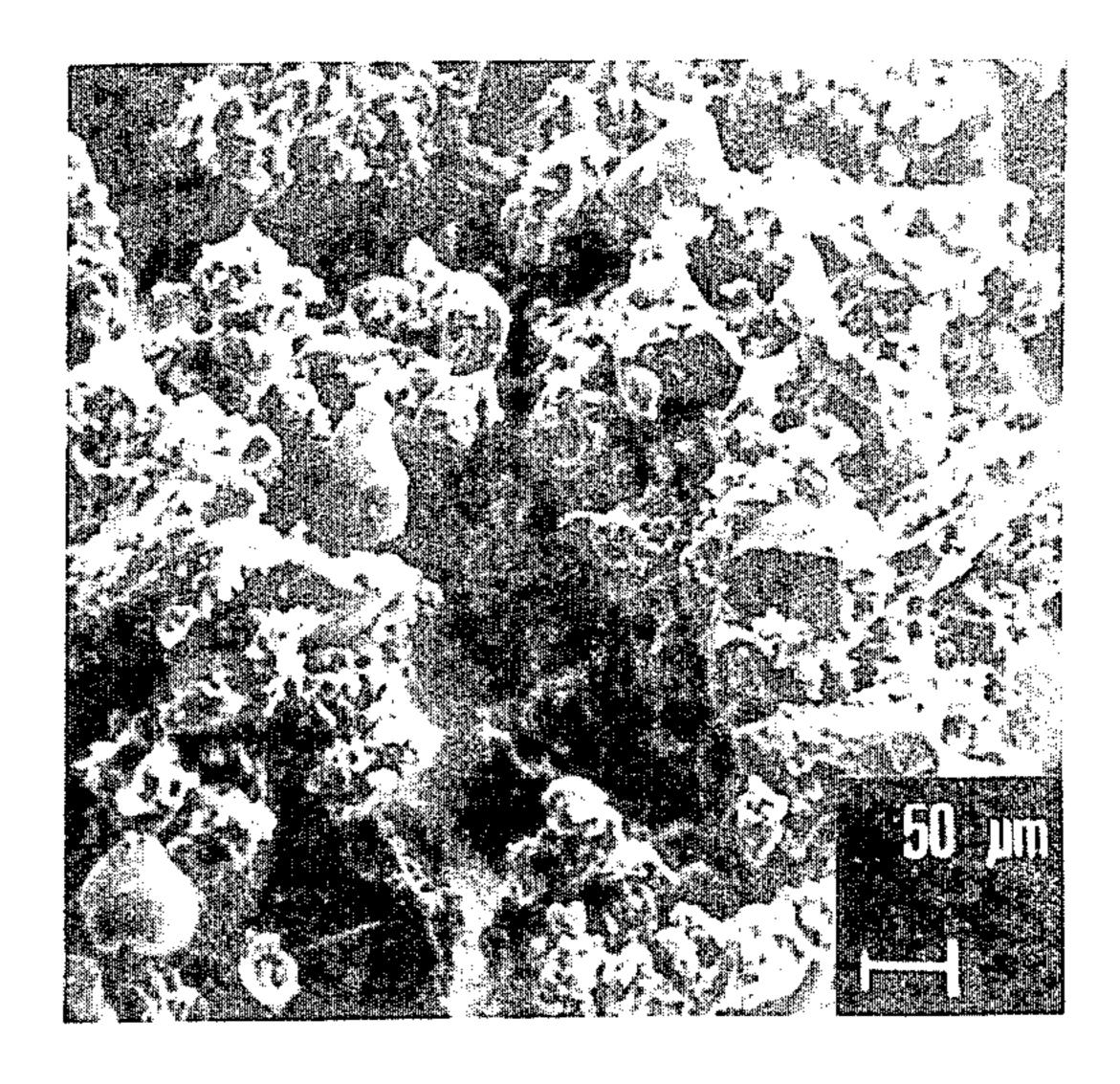
Electron micrograph of new car tyre buffings.
