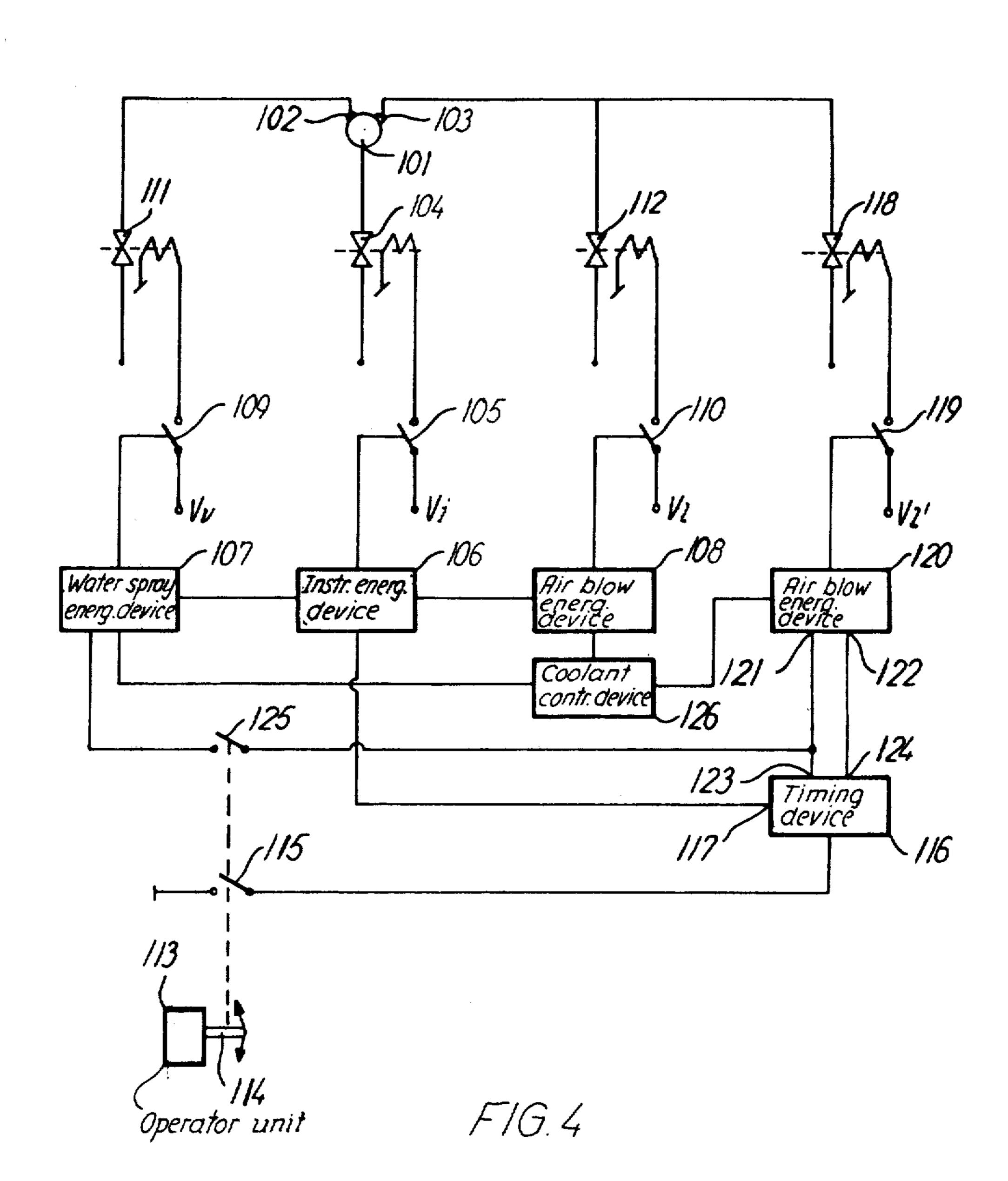
DENTAL APPARATUS WITH A NUMBER OF DENTAL INSTRUMENTS CONNECTED TO A COMMON CONTROL CIRCUIT AND A COMMON OPERATOR UNIT
