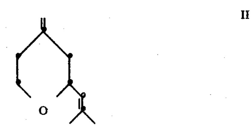
is hydrogenated over a platinum dioxide or platinum/-charcoal catalyst in the presence of a strongly acidic cation exchanger. The product is a useful fragrance material which also occurs naturally and is known as rose oxide.
