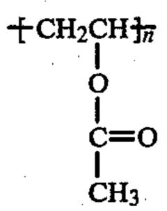
The preferred amount of EVA introduced into the asphalt flux ranges from about 1 weight percent to about 10 weight percent. The more preferred amount of EVA is 5% by weight EVA to 95% by weight asphalt flux.
