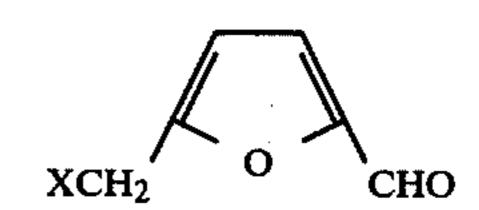
wherein X is Cl or Br, which comprises carrying out a acid-decomposition of saccharide in a water/organic solvent/magnesium halide system with hydrochloric acid, sulfuric acid, hydrogen chloride or other mineral acid in the presence or absence of surface active agent as a catalyst. The 5-halomethylfurfural is useful as an intermediate of medicines, agricultural chemicals, perfumes and the like.
