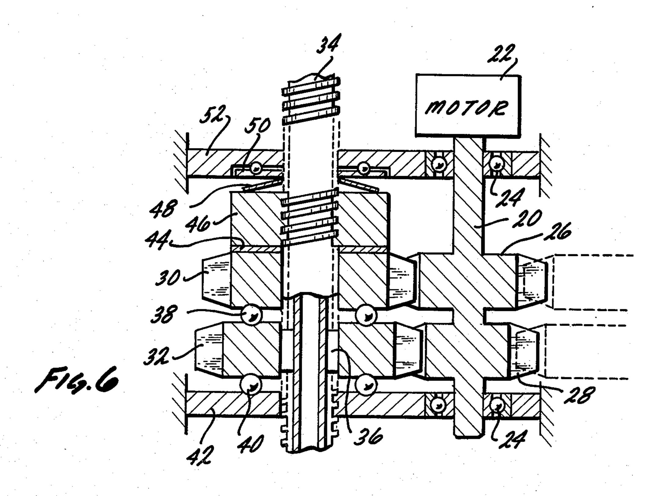
This invention relates to apparatus for producing 5 penetrations in the sidewalls of boreholes in oil wells for augmenting oil flow. The invention further relates to apparatus for producing a number of such penetrations simultaneously. The invention is particularly concerned with producing "clean" holes which are sharply defined 10 and which do not have any contamination creating subsequent difficulties.
