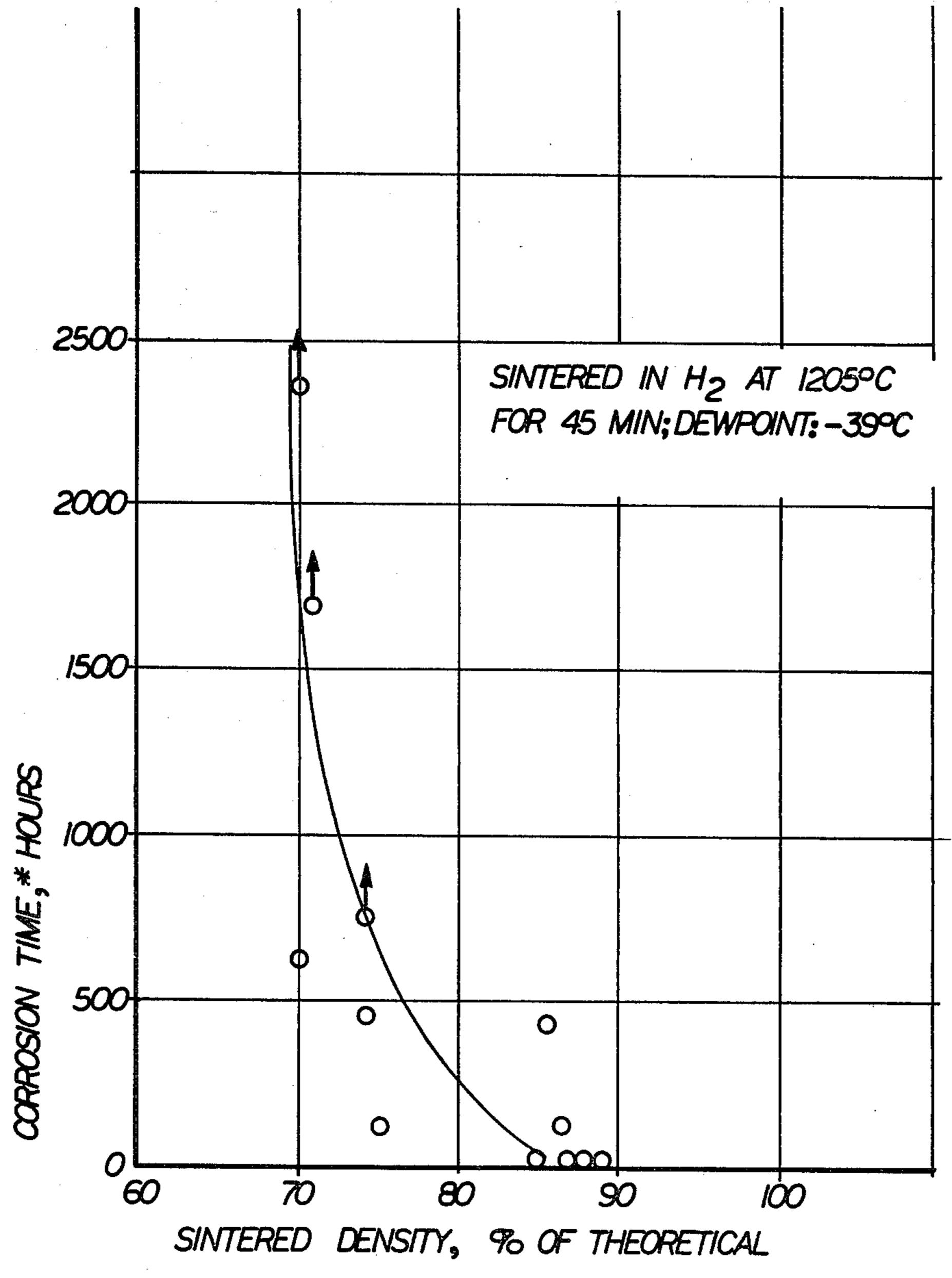
\* TIME AT WHICH CORROSION FIRST APPEARS IN 59% AQUEOUS NaCI
