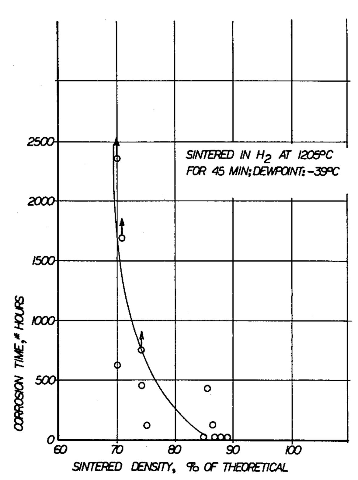
\*TIME AT WHICH CORROSION FIRST APPEARS IN 596 AQUEOUS NaCI
