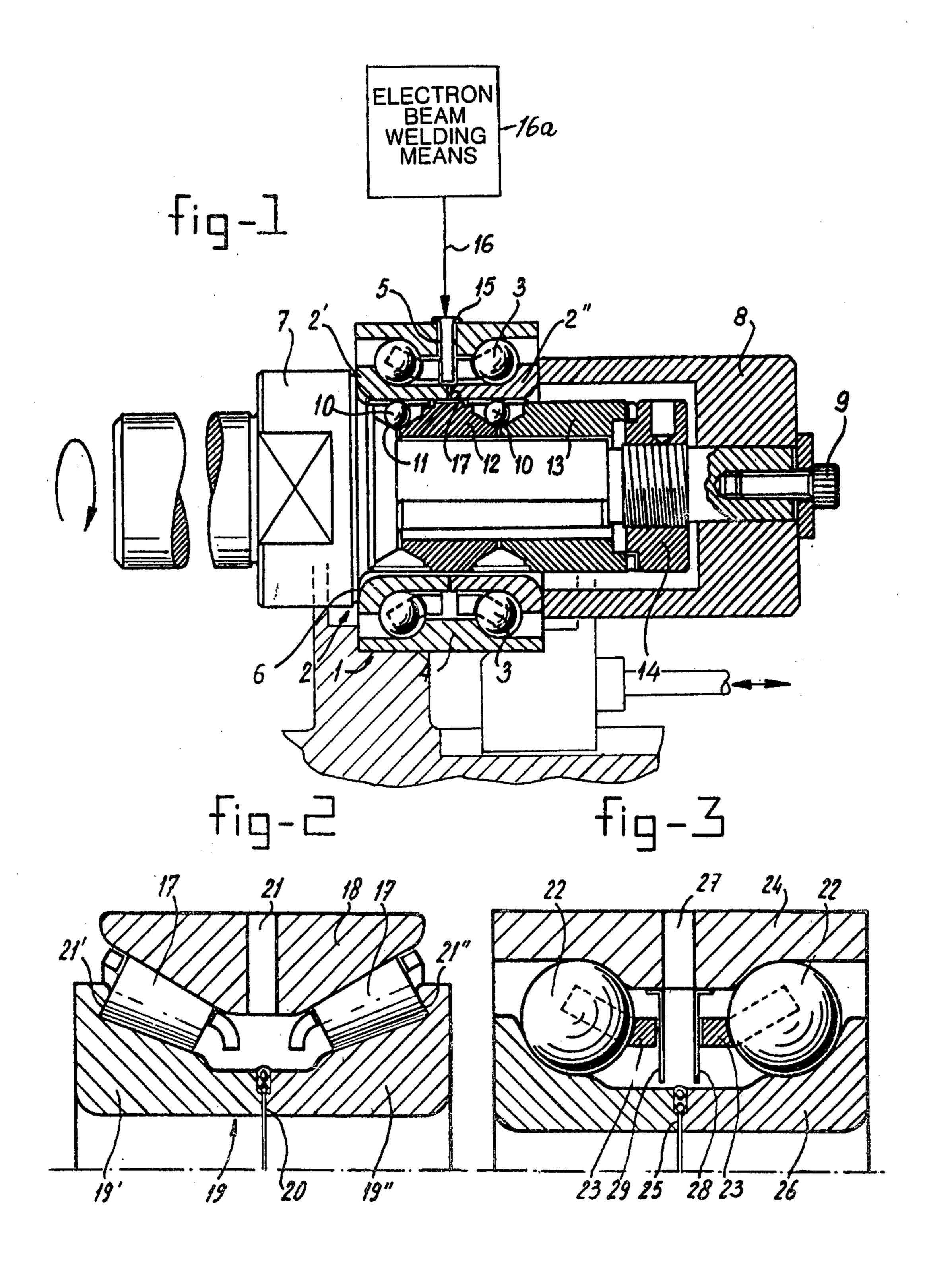
DEVICE FOR PRODUCING AN OBJECT CONSISTING OF AT LEAST TWO PARTS MOVABLE RELATIVE TO ONE ANOTHER ONE OF WHICH IS SUBSTANTIALLY ENCLOSED WITHIN THE OTHER
