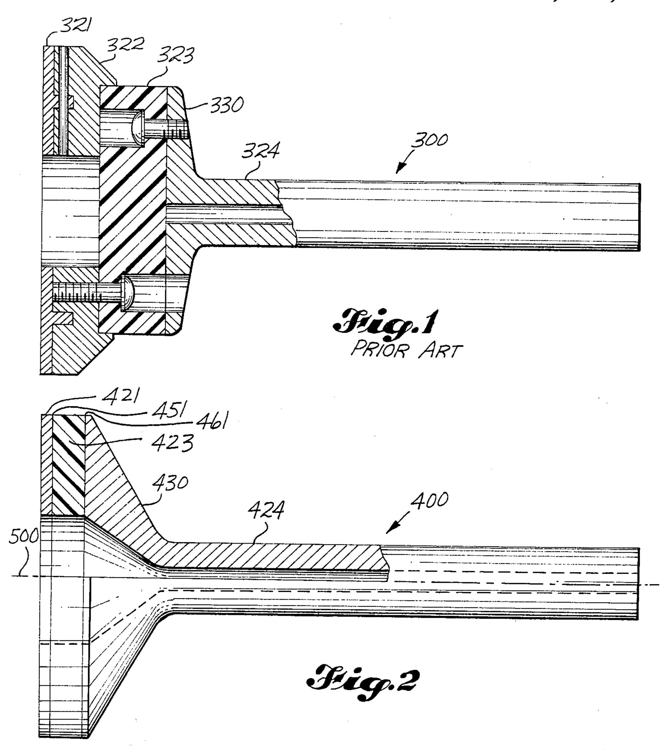
RAM ASSEMBLY FOR ELECTROMAGNETIC RIVETER
