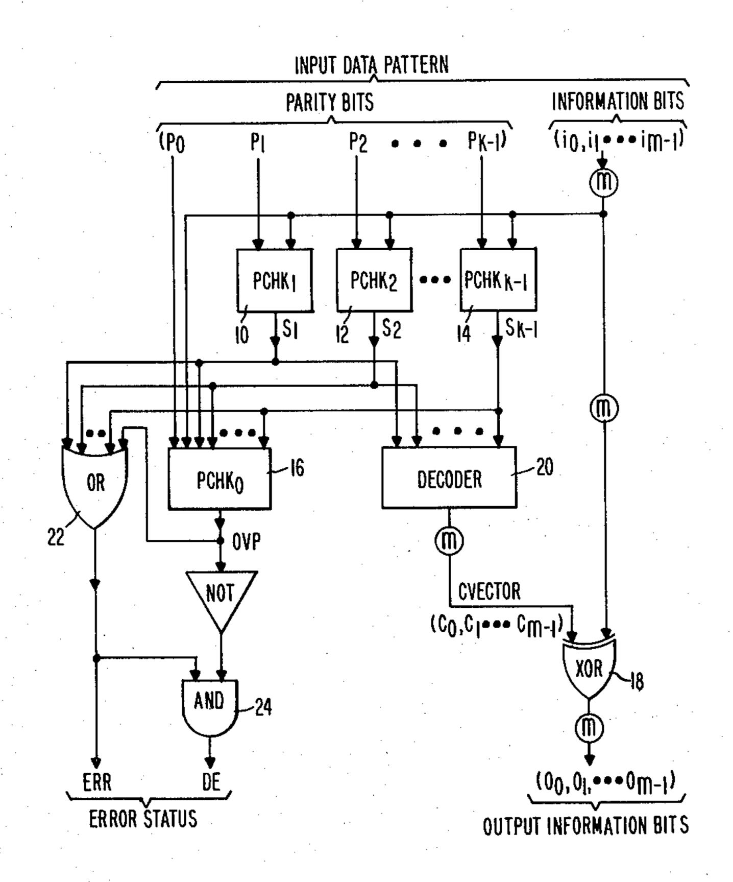
INPUT DATA PATTERN PARITY BITS INFORMATION BITS (io,ii.•••im-1) (P0 Fig.1 ••• PCHK K-1 PCHK! PCHK2 SK-1 PCHK<sub>0</sub> DECODER OR OVP TON CVECTOR XOR AND ERR ERROR STATUS OUTPUT INFORMATION BITS
