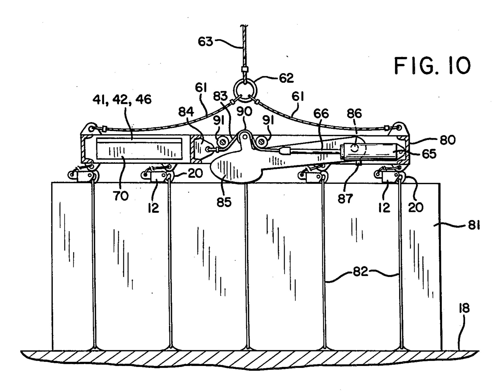
PNEUMATIC RELEASE FOR LOAD HOOK
