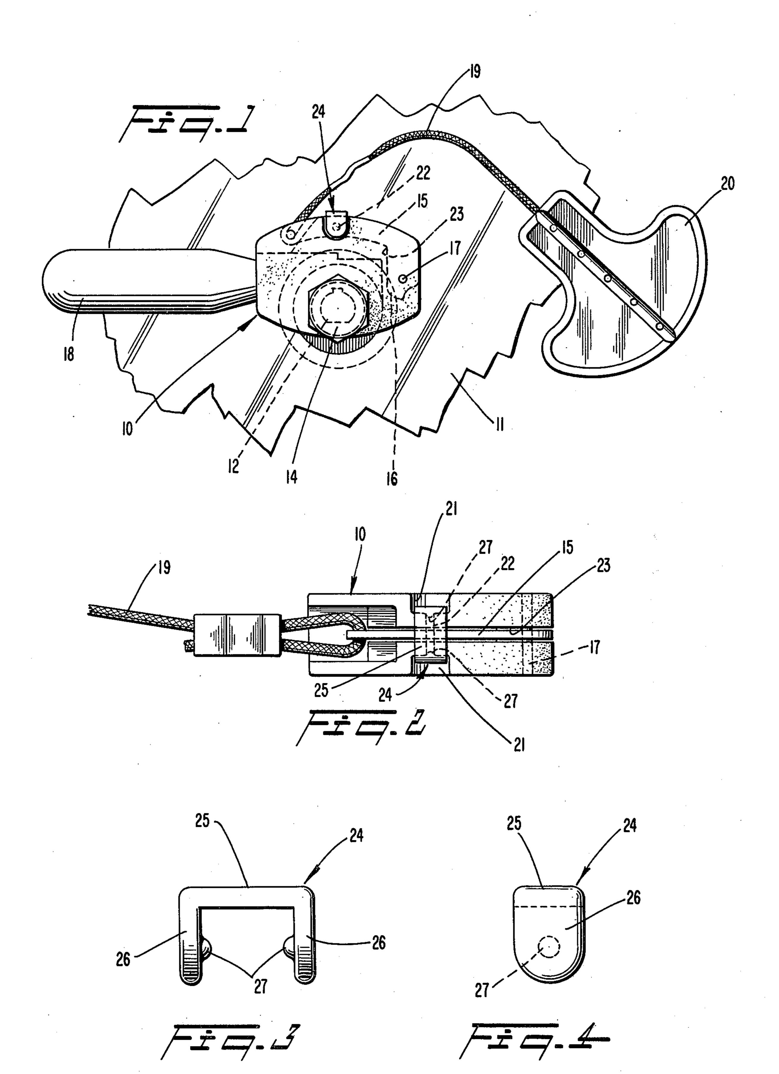
to a portion 11 of the side wall of an inflatable article, there being a stem generally shown at 12 sealed to the side wall 11, such stem extending through the inflator 10 and secured and sealed thereto by a cap nut 14.
