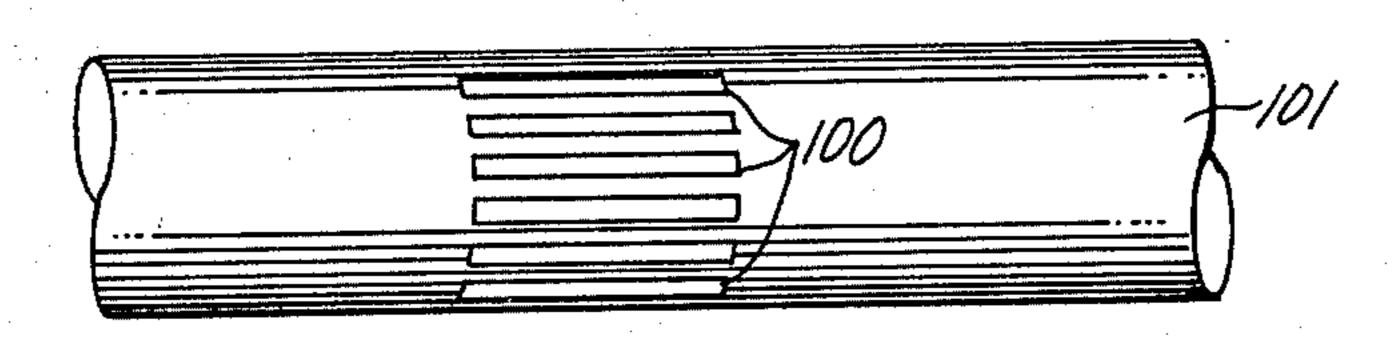
of twisting displacement of the shaft. A sensor detects changes in magnetization of the zone.
