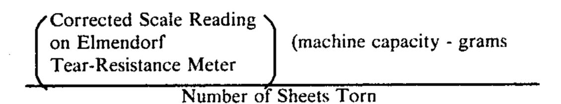
The Elmendorf Tear-Resistance Meter is described in ASTM Standard No. D 1922.
