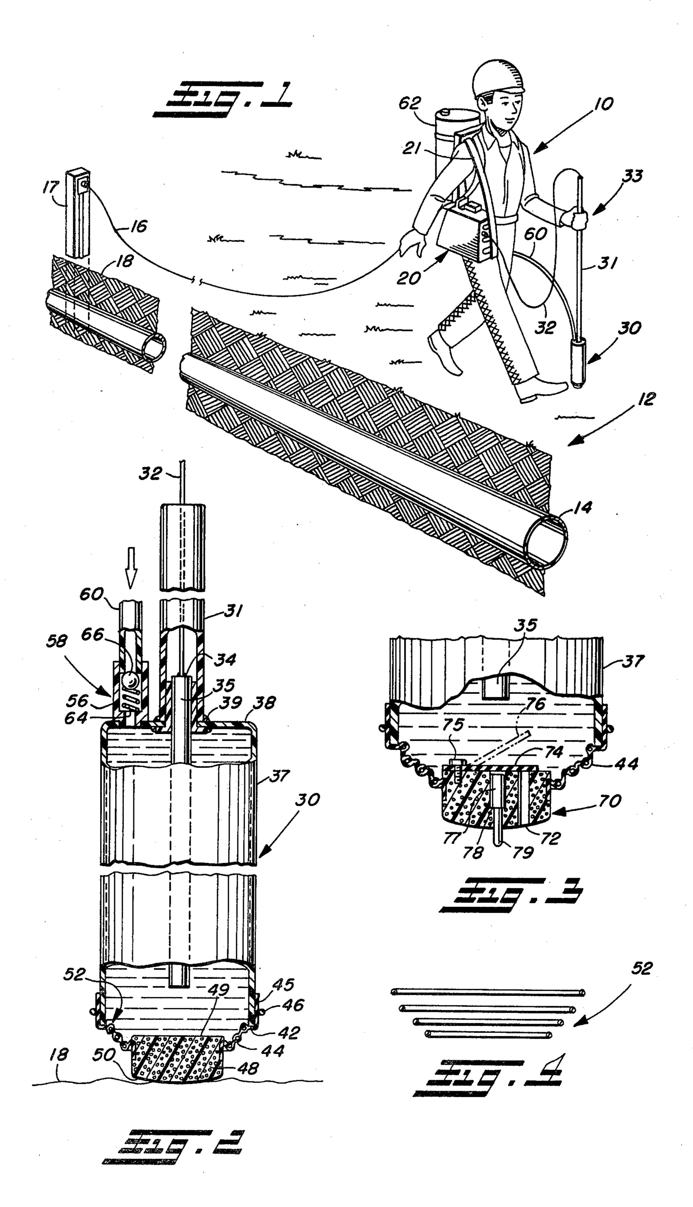
LOW RESISTANCE, FLUID REPLENISHING, REFERENCE CELL AND METHOD FOR USING SAME IN STRUCTURE-TO-SOIL ELECTRICAL **SURVEYS**
