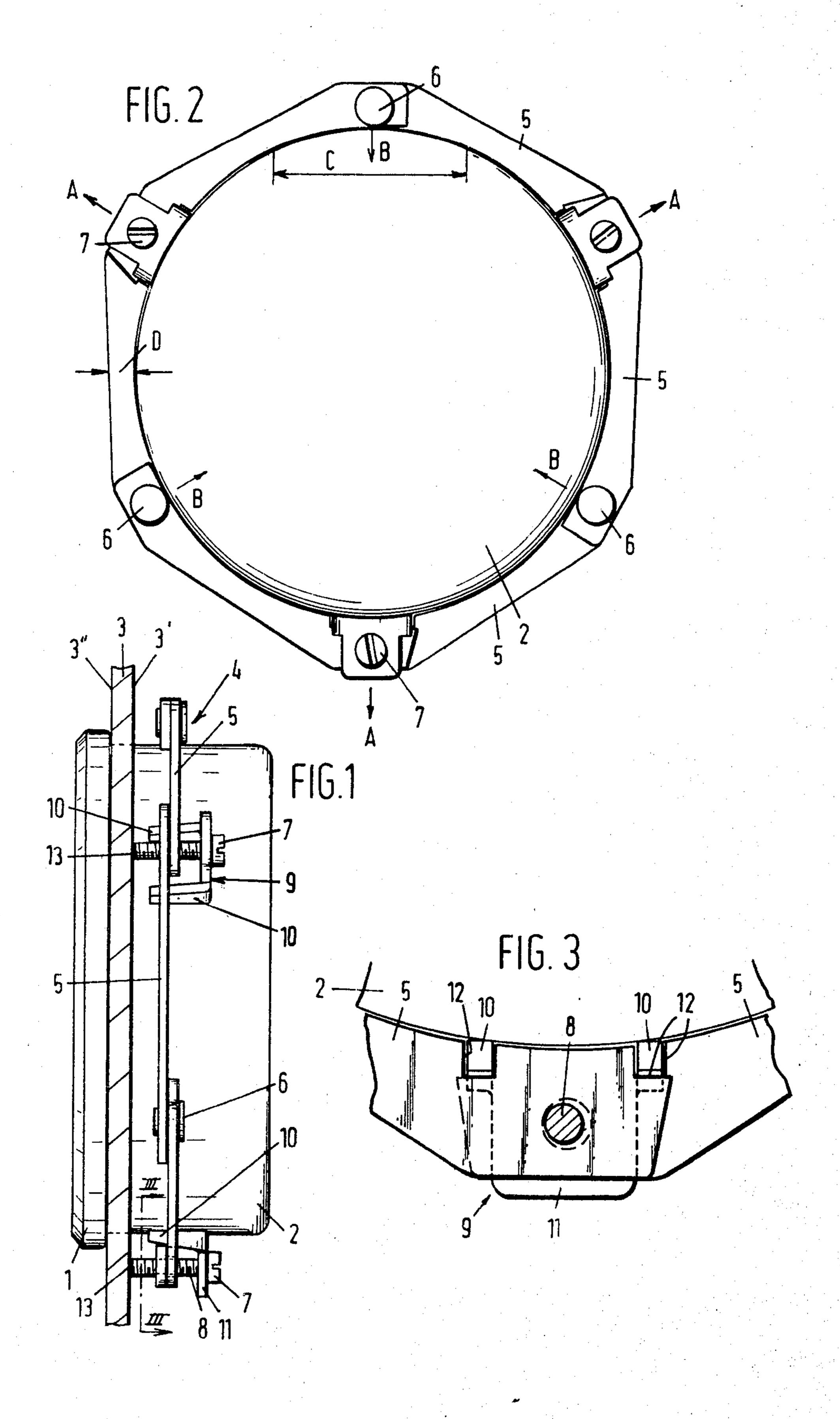
The invention relates to an attachment means for an article recessed in a wall element, in particular an article projecting through an opening in a panel, said 5 attachment means, through engagement on a part of the article projecting on the other side of the panel, in cooperation with stopping devices acting on the panel, being adapted to fix the article in a stationary axial position relative to the panel.
