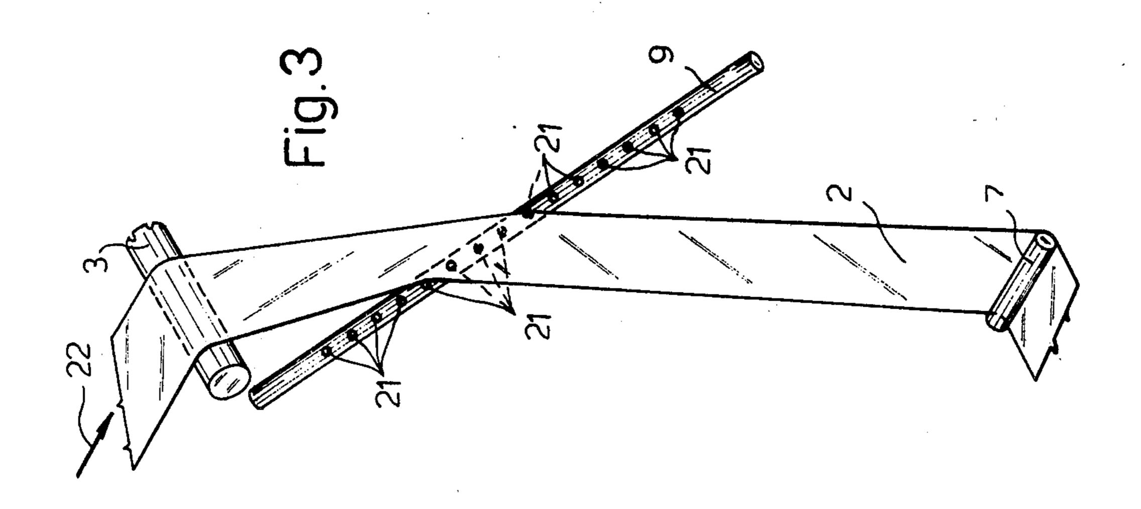
DEFLECTOR AND INVERTER DEVICE FOR STRIPS OF WEB MATERIAL
