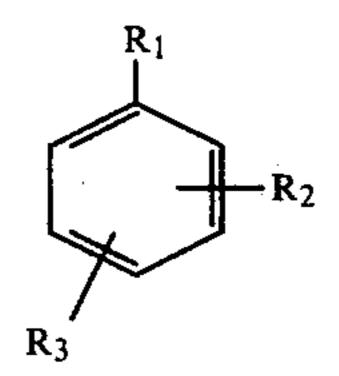
wherein R<sub>1</sub>, R<sub>2</sub> and R<sub>3</sub> respectively represent hydrogen atom, C<sub>1</sub>-C<sub>5</sub> alkyl group and chlorinated derivatives thereof as a side reaction inhibitor at a ratio of at least 0.001 wt. % in the reaction medium.
