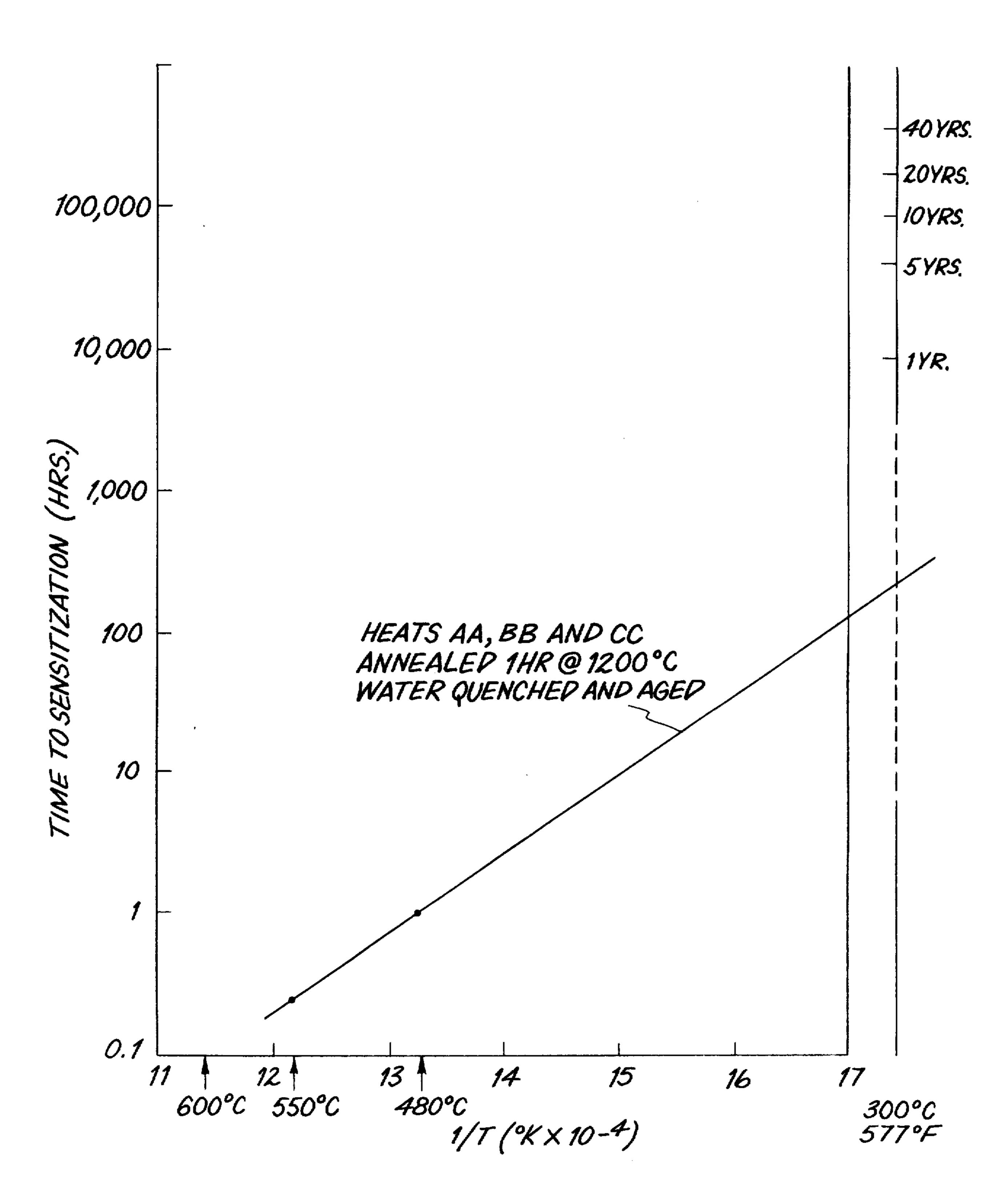
METHOD OF MAKING TITANIUM-STABILIZED FERRITIC STAINLESS STEEL FOR PREHEATER AND REHEATER EQUIPMENT APPLICATIONS
