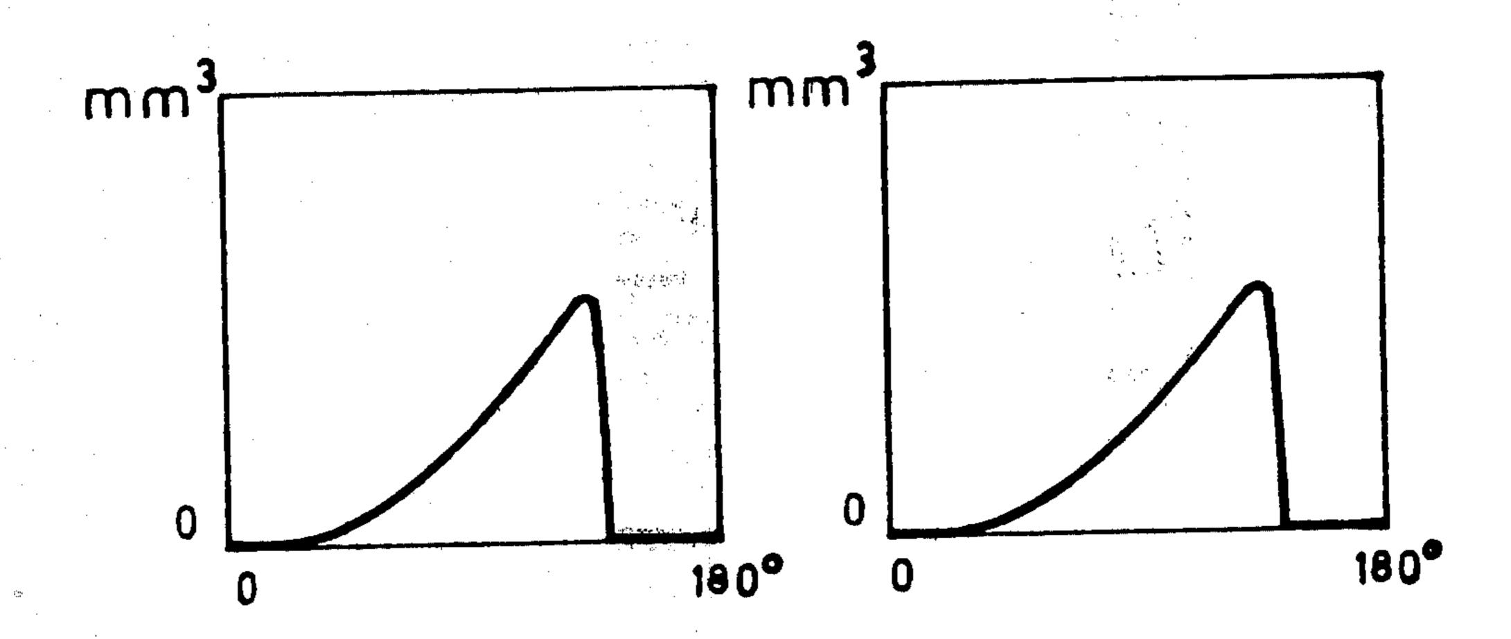
Air pump delivery curve
