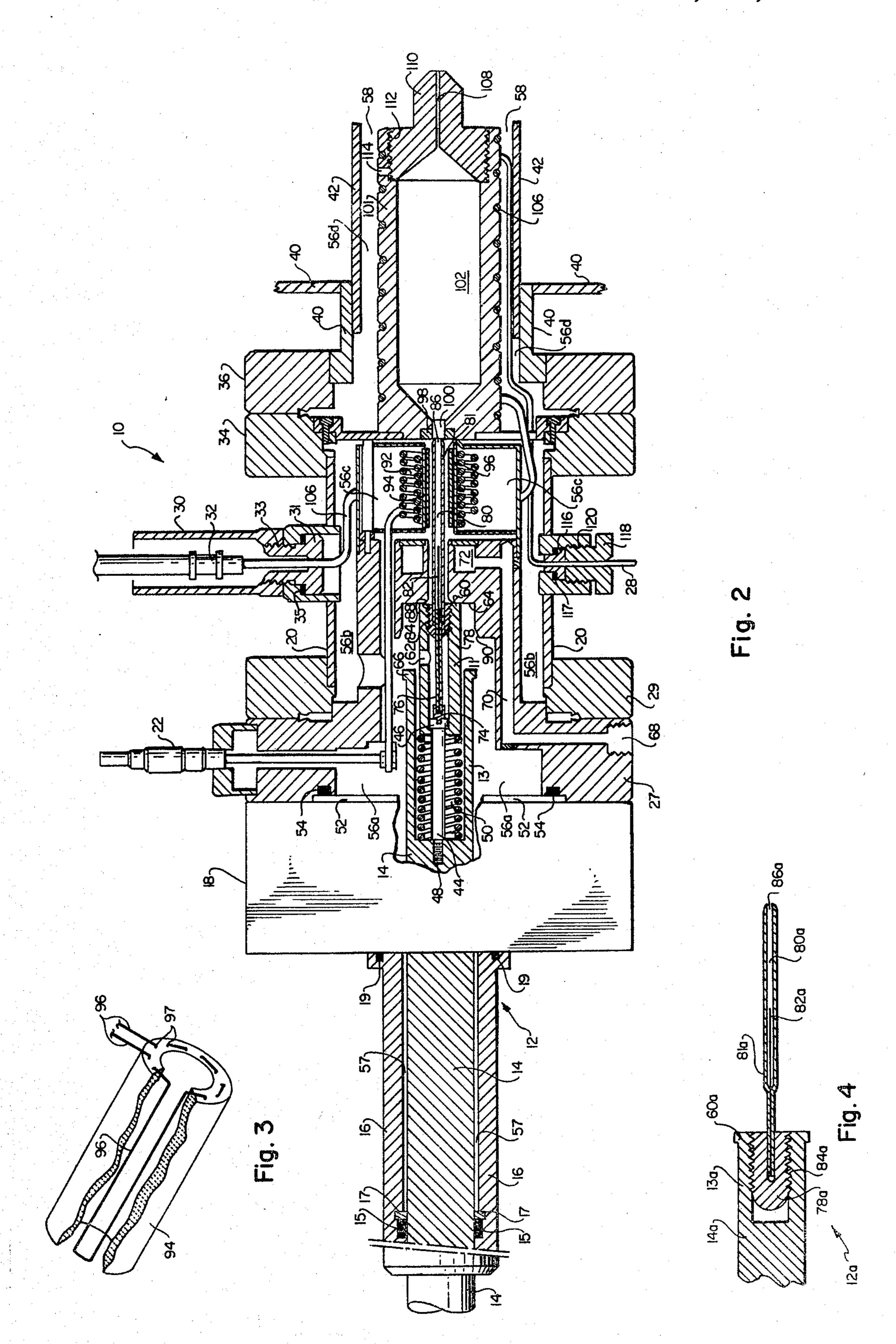
ter. This type of pyrolysis apparatus allows the scientist to obtain mass spectra of the individual components of the pyrolyzed sample produced at different times during pyrolysis, since the volatile pyrolysis products are not mixed and delayed in an expansion chamber. How- 5 ever, highly volatile components produced in this type of pyrolysis apparatus often escape analysis by the mass spectrometer due to the minimum response time required by the mass spectrometer for analysis thereof.
