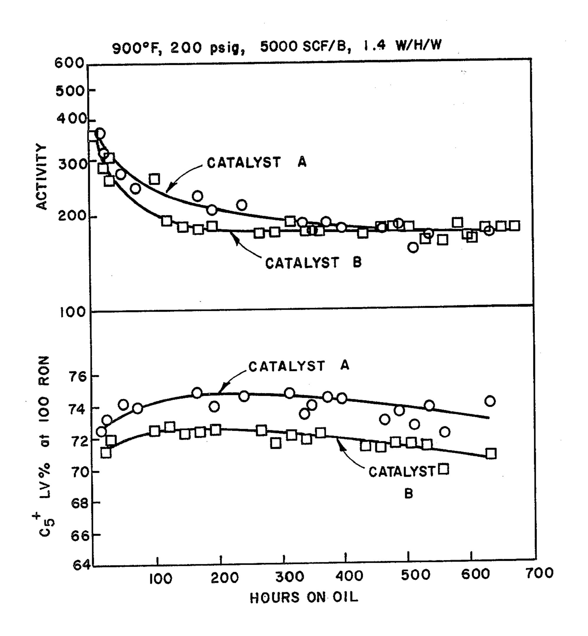
FIGURE 2 REFORMING LOW SULFUR PARAFFINIC NAPHTHA WITH Pt-Ir-Se
