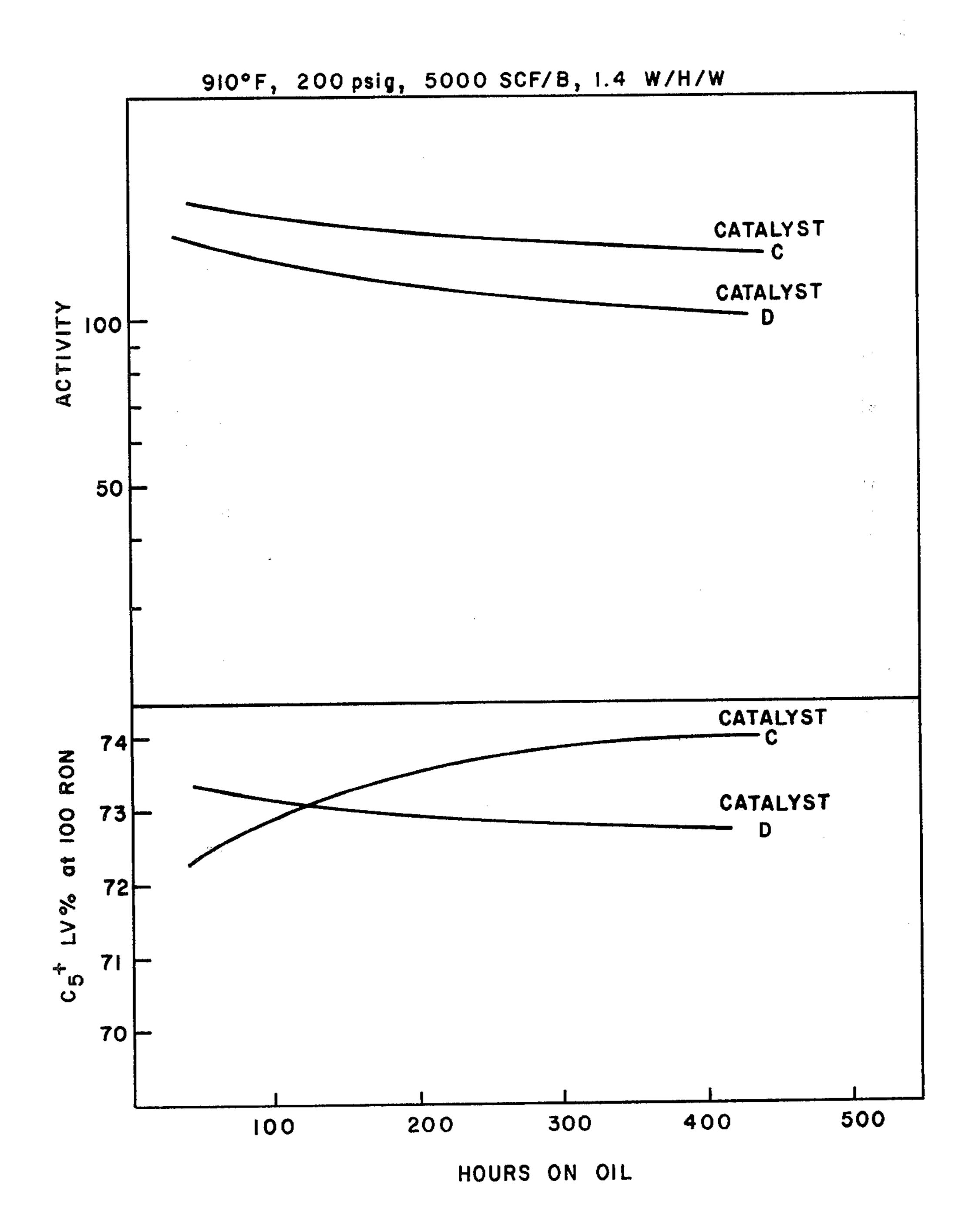
FIGURE 3 CYCLIC REFORMING OF LOW SULFUR PARAFFINIC FEED WITH Pt-Ir-Se
