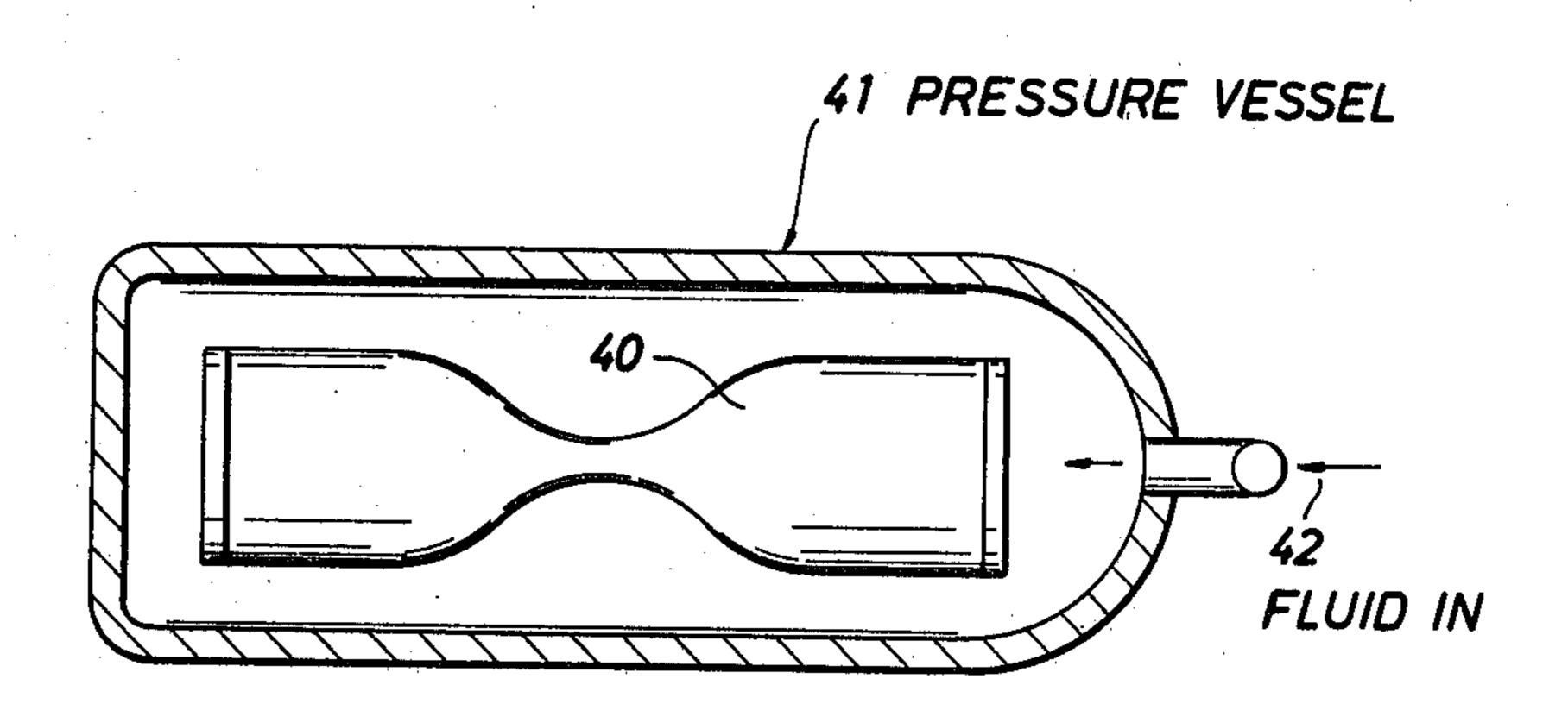
B. PLACE PIPE IN PRESSURE VESSEL AND PROPAGATE BUCKLE SOMEWHAT FURTHER BY PUMPING HYDRAULIC FLUID (OR WATER) INTO THE VESSEL. NOTE THE PRESSURE REQUIRED TO PROPAGATE THE BUCKLE: THIS WILL BE RELEASE PRESSURE OF THE RELEASE MECHANISM.
