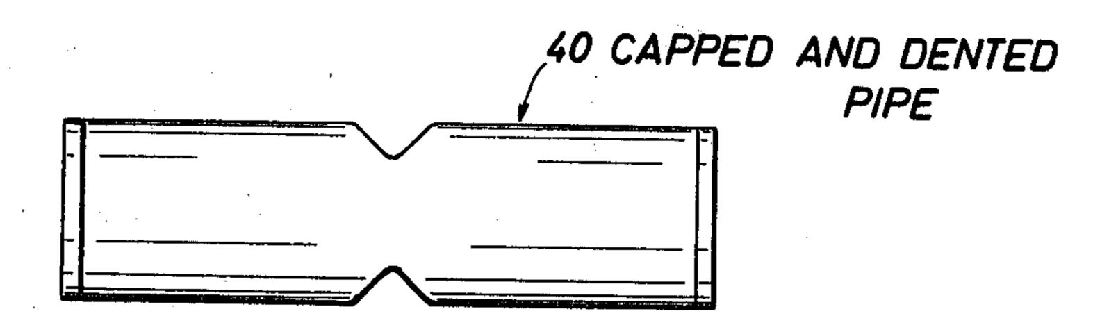
A. MECHANICALLY DENT THE CENTER OF A CAPPED, STUB PIPE.
