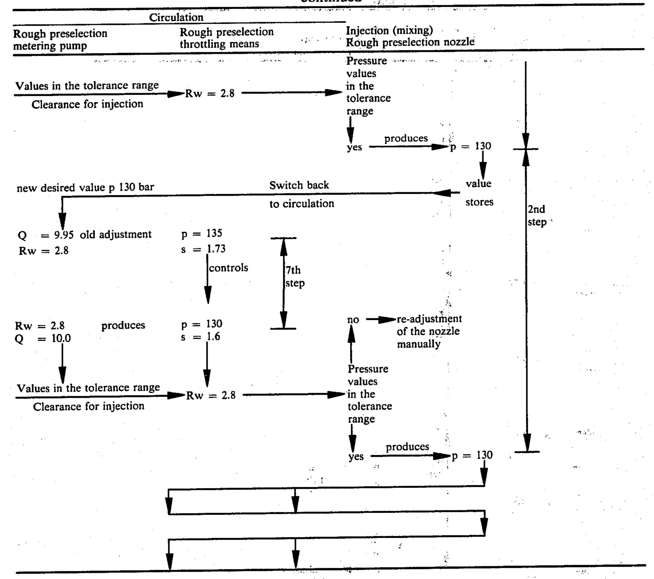
As shown by the circulation control steps, a value of Q=10.0 kg/min and p=148 bar, which lies within the permitted deviations, has been adjusted after the 4th control step.
