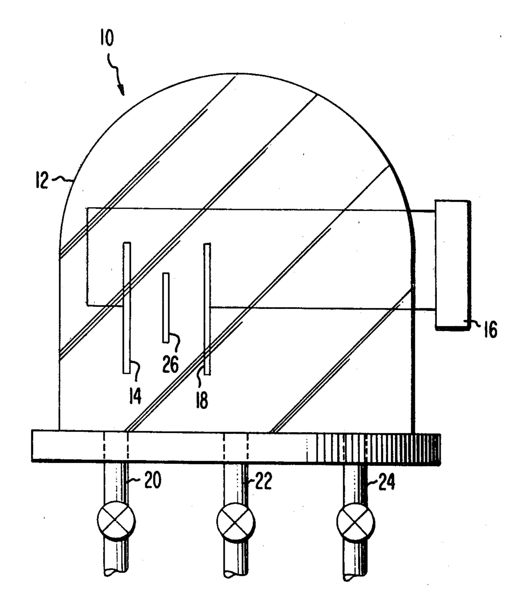
This invention relates to a method of depositing by glow discharge techniques a low surface energy layer 5 on a substrate. More particularly this method relates to the preparation of a low surface energy film having improved adhesion to the substrate.
