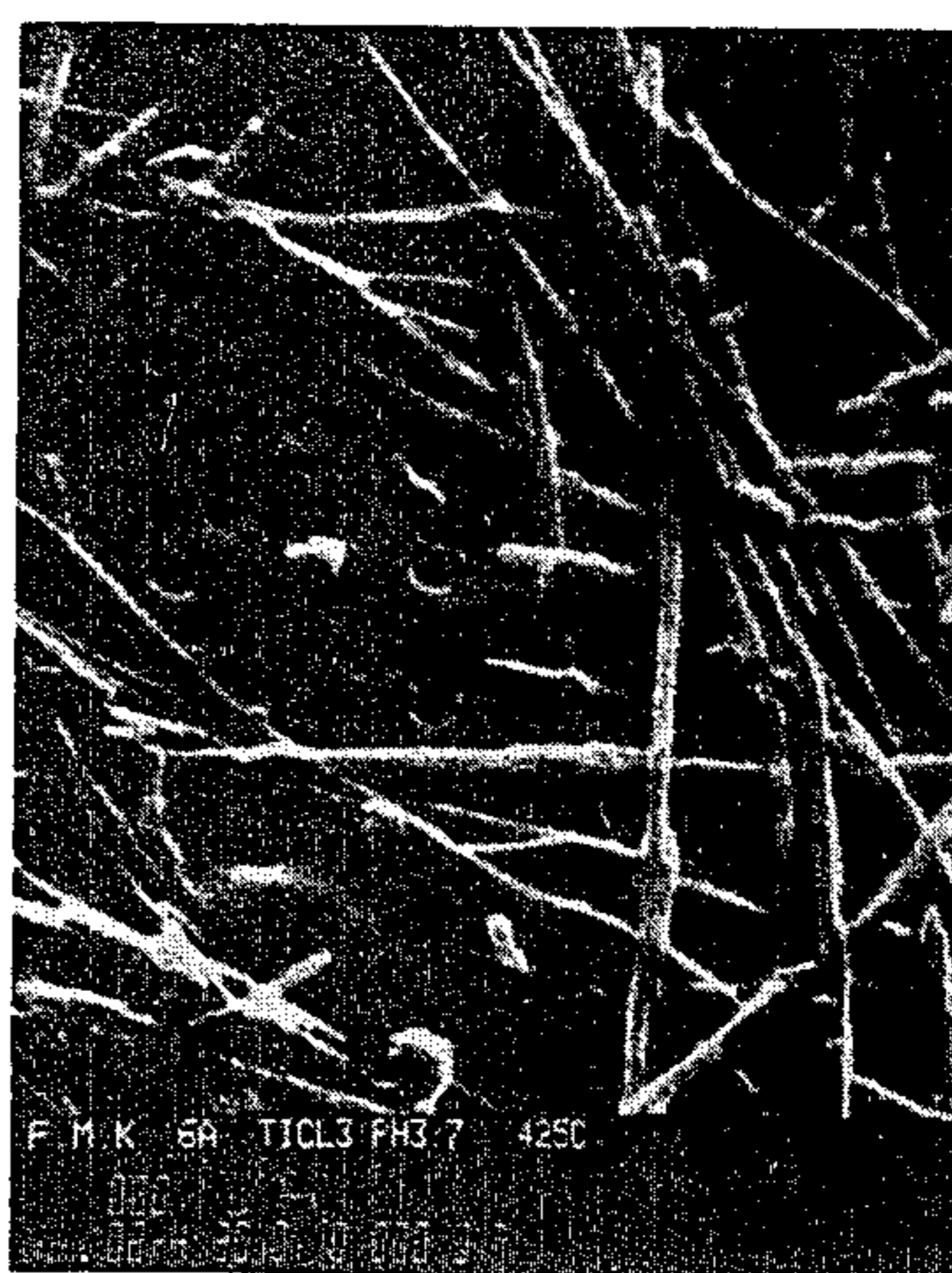
Fig. 7 Chrysotile asbestos modified as in Example 1D
