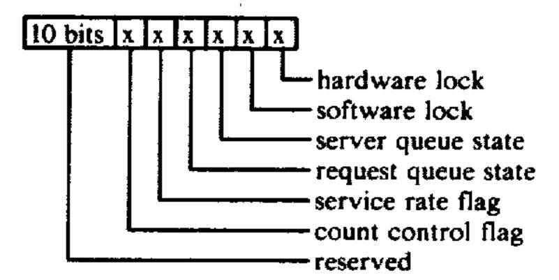
The port locks are used by the processes or processors to give one process exclusive access to the port during insertion or removal operations. The queue state flags indicate whether the associated queues are empty or occupied.
