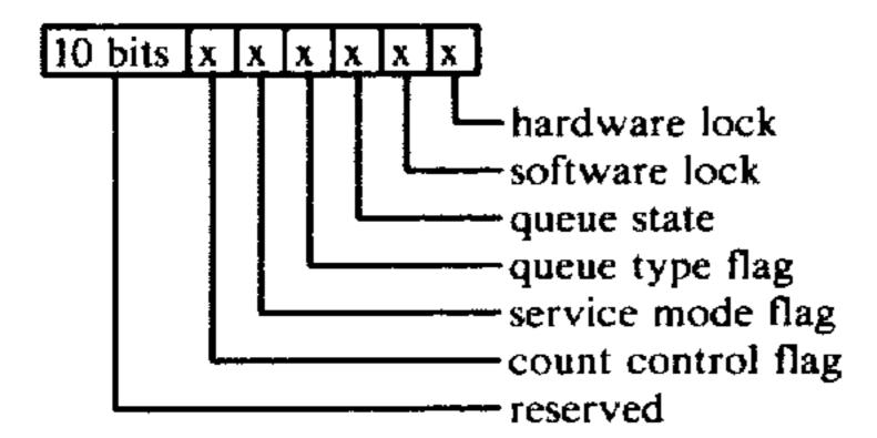
The port locks are used to give one processor or one process exclusive access to the port during insertion or removal operations. When the port is locked by a processor, the second double byte of the port control segment (152) contains the locking processor's identification value. When the port is locked by a process, the second double byte contains the locking process's identification value.
