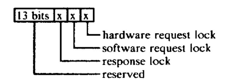
The request locks and the response lock must be clear before transmission begins. At the onset of communication, one of the request locks and the response lock are set. Following the communication, the request lock is cleared, with the response lock left set until the processor carries out the functions requested by the message.
