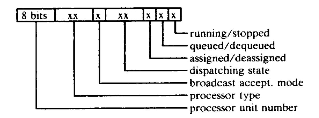
The processor unit number is the value loaded into the processor at initialization or reset.
