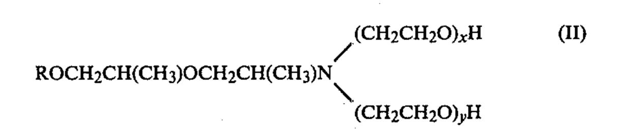
wherein R is an alkyl group containing 10 to 12 carbon atoms; x and y are integers, the sum of which is from 2 to about 20. The aqueous acid plating baths of the invention will preferably contain as a brightening agent, at least one carbonyl-containing compound. These plating baths exhibit low foaming characteristics.
