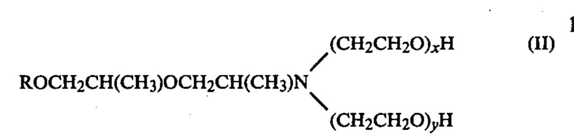
wherein R is an alkyl group containing 10 to 12 carbon atoms; x and y are integers, the sum of which is from 2 to about 20. The aqueous acid plating baths of the invention which each preferably contain as a brightening agent, at least one carbonyl-containing compound, exhibit low foaming characteristics.
