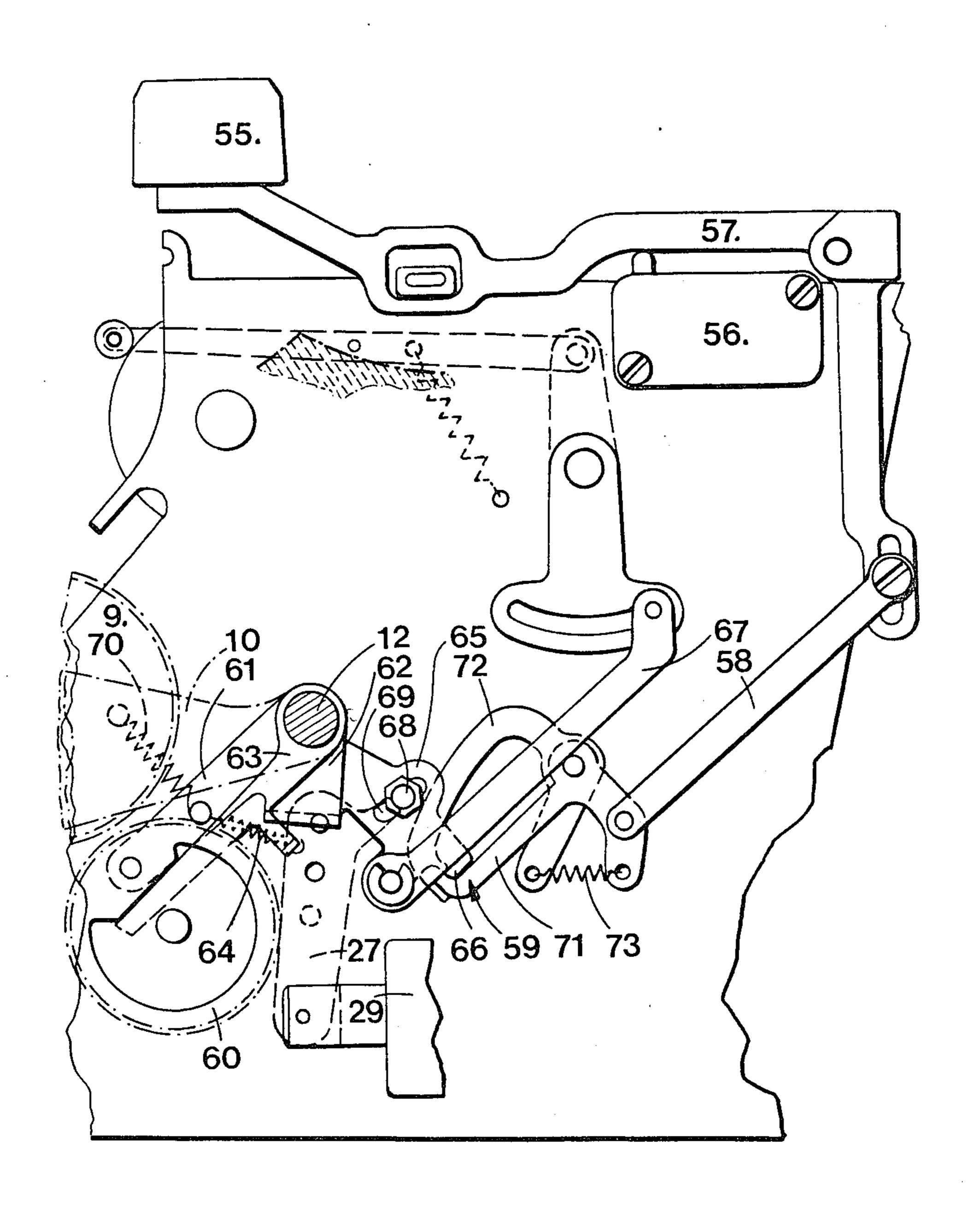
In known typewriters, the driving of the platen is effected by a ratchet wheel for the small angular dis- 5 placements corresponding to the interline spacing and by a motor rotating continuously, via gears, for the larger angular displacements corresponding to the introduction or ejection of paper.
